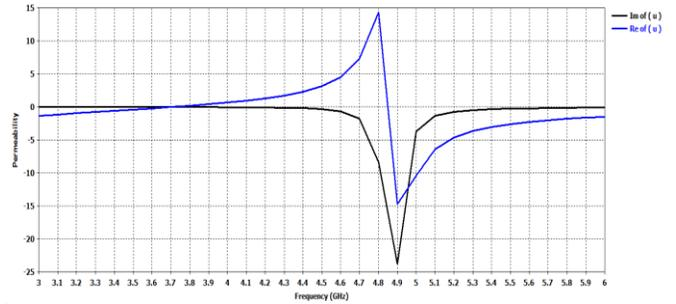
Fig. 9. Effective complex permeability values of the BS-SRR unit cell.
