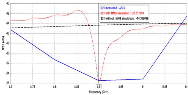
Fig. 12. Measured  $S_{21}$  with and without employing the MNG.
