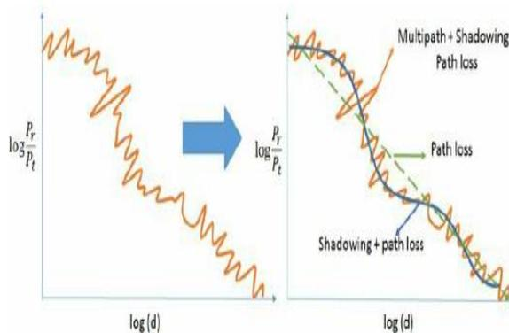
Figure. 1 Path Loss, Shadowing and Multipath versus Distance [2].
