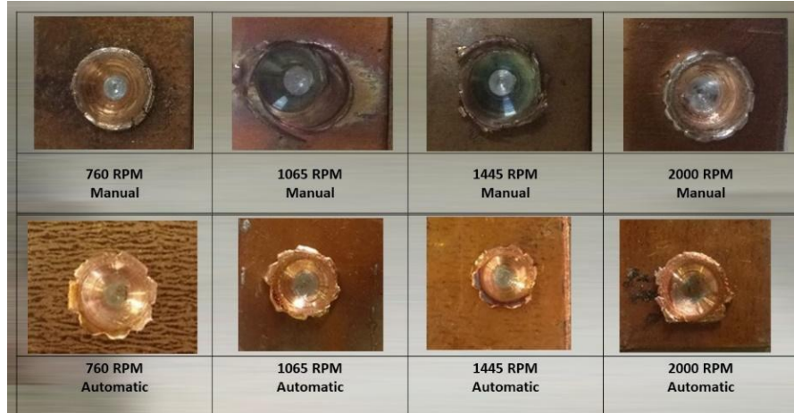
Figure 6. The shape of friction stir spot welded point
