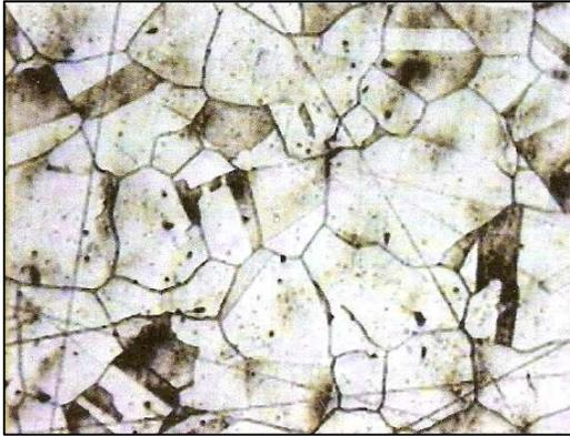
Figure (3) Microstructure of carbon steel before subjected to annealing treatment
