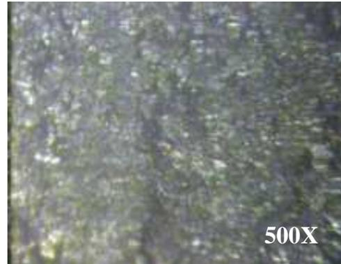
Figure (6) Microstructure of carbon steel after subjected to hardening treatment cooling in oil solution
