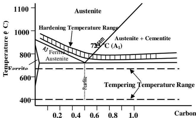
**Figure (1) Temperature Range for Tempered And Hardened Types of Carbon Steel [4]**
