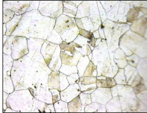
Figure (4) Microstructure of carbon steel before subjected to hardening treatment
