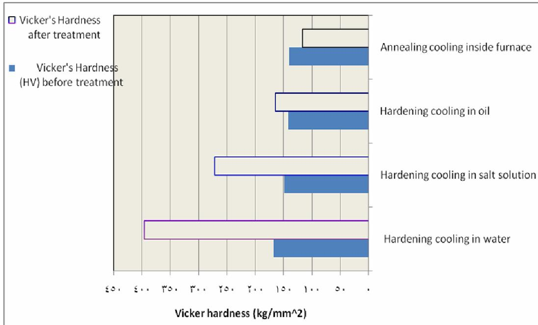
Figure (2) Mean of Vicker's Hardness tests
