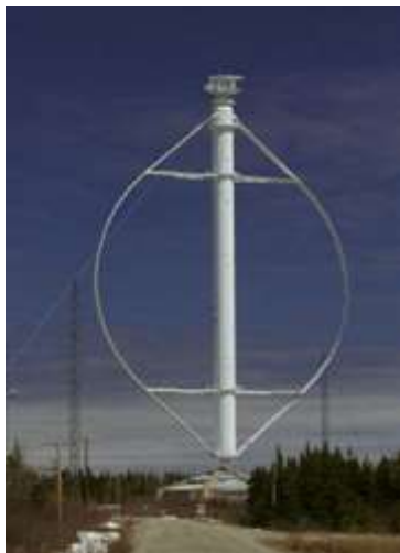
Fig. 1: a photo of a vertical axis wind turbine
