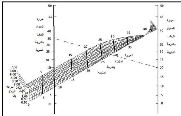
Fig. 2. Calculation ET directory values using temperatures, dry thermometer and wet thermometer and wind speed.
