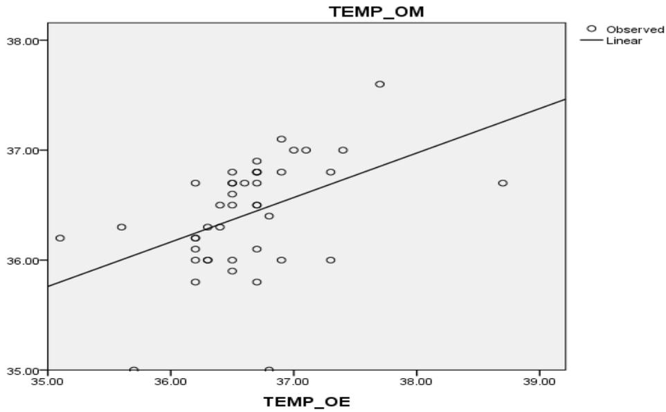
(B) Correlation between oral-electronic and oral-mercury methods in measurement of temperature ( $r = .448$ ,  $P < 0.001$ )
