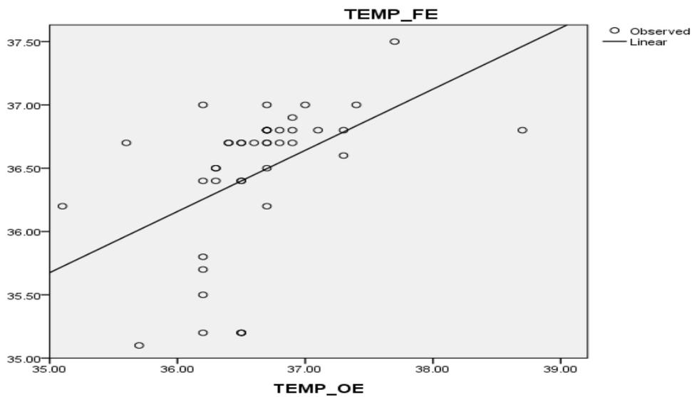
(C) Correlation between forehead-electronic and oral-electronic methods in measurement of temperature ( $r=.469$ ,  $P < 0.001$ )
