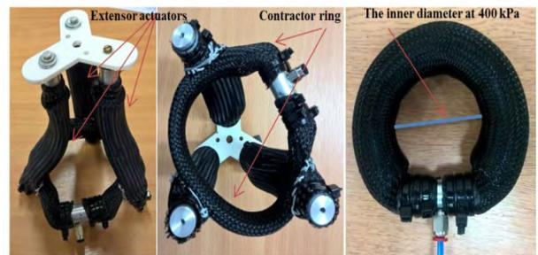
FIGURE 17. The structure of the extension-circular gripper.
