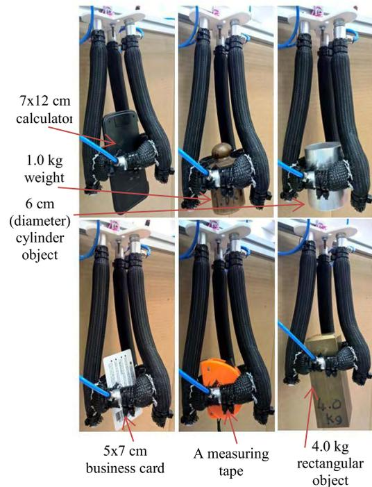
FIGURE 20. Multiple objects grasped by the extension-circular gripper.
