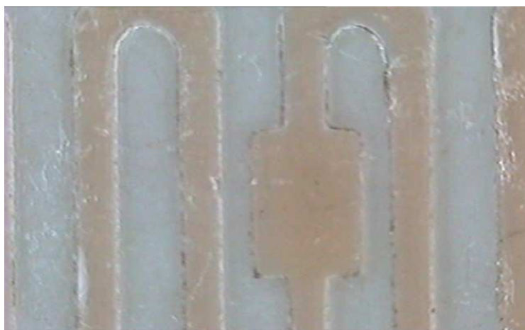
Fig.5, Fabricated master mould showing two micro channels chamber
