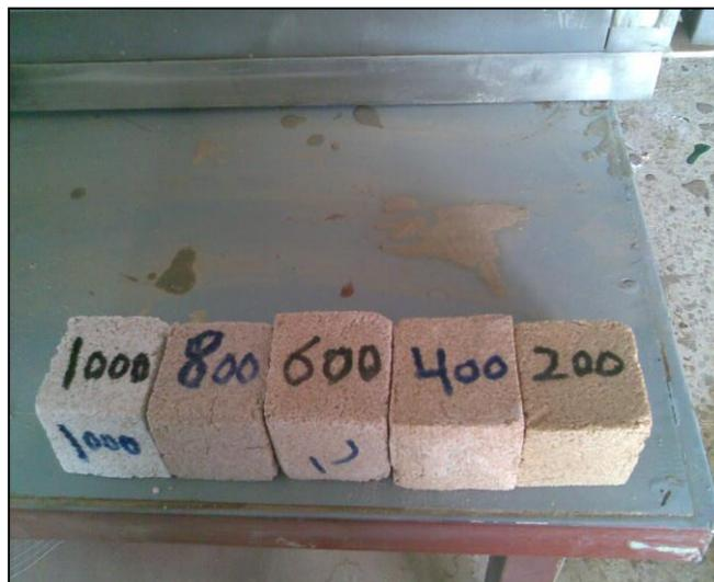
**Fig.(2): Change color of samples with a high temperature**
