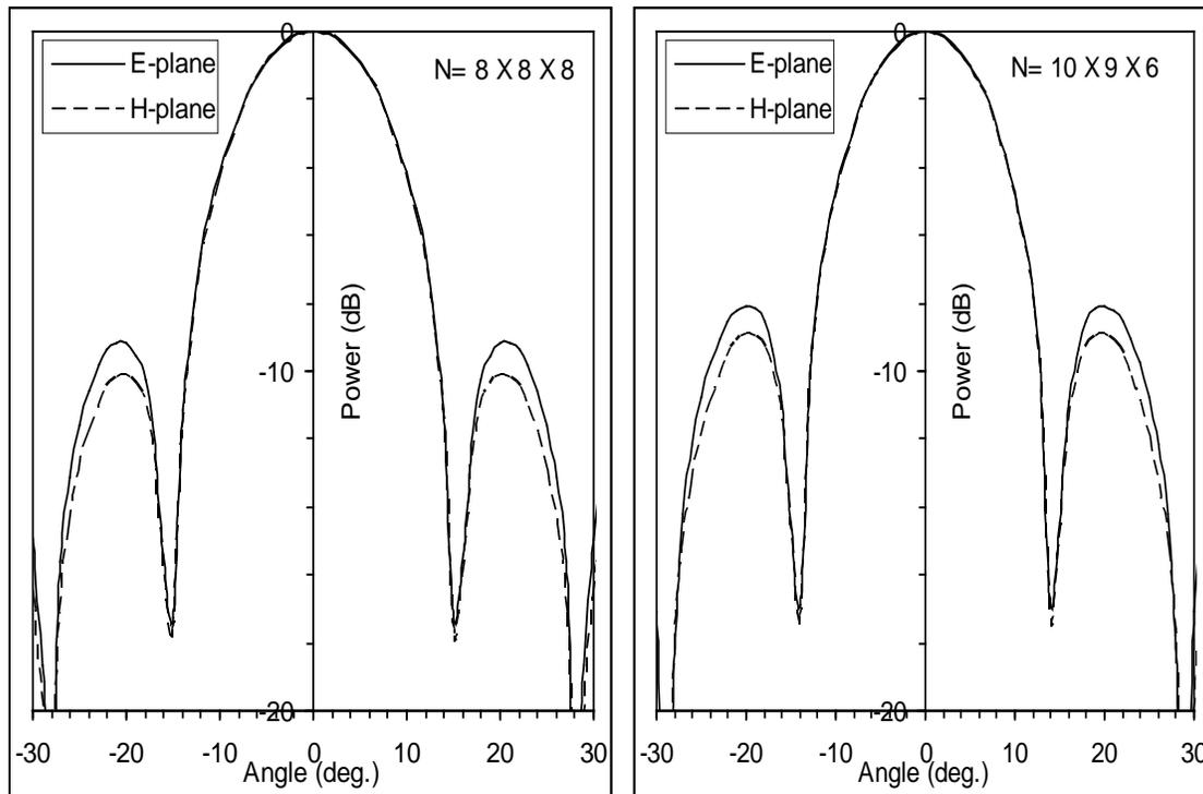
**Fig.(7) : Radiation patterns of special arrangement of elements for circular polarization case.**
