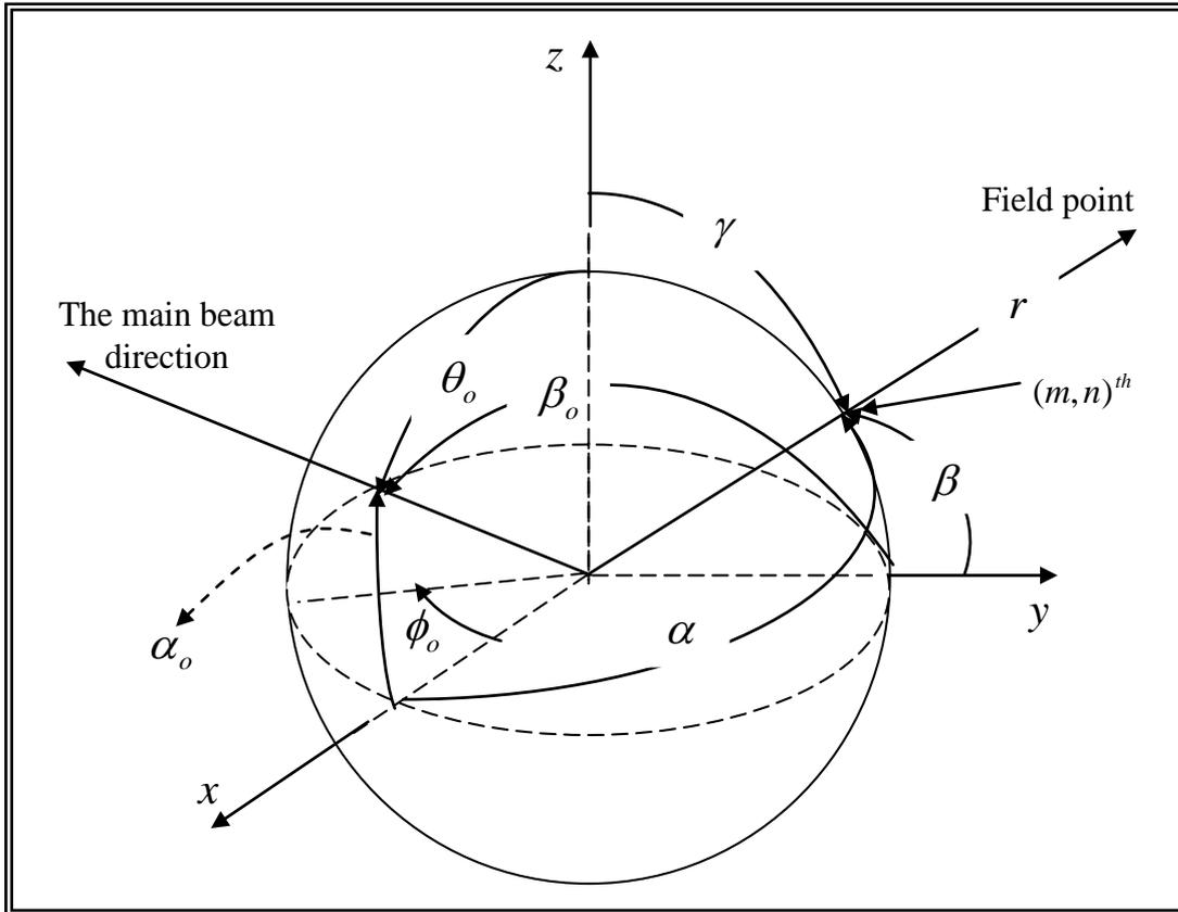
**Fig.(1) : Spherical polar coordinate system and direction angles of spherical arrays.**
