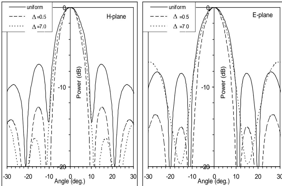
**Fig.(9) : Comparison of radiation pattern of a uniform spherical array with :  $\Delta$**
