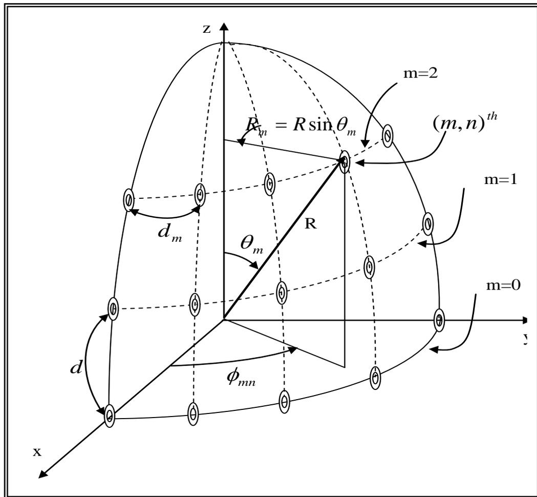
Fig.(2) : Spherical array geometry .
