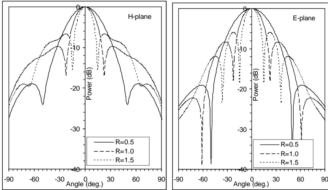
**Fig.( 5) : Radiation patterns of a uniform spherical array ( $m = 0$ ) of five ARMSA elements with  $(R = 0.5\lambda, d = 0.016\lambda), (R = 1.0\lambda, d = 0.64\lambda)$  and  $(R = 1.5\lambda, d = 1.27\lambda)$  .**
