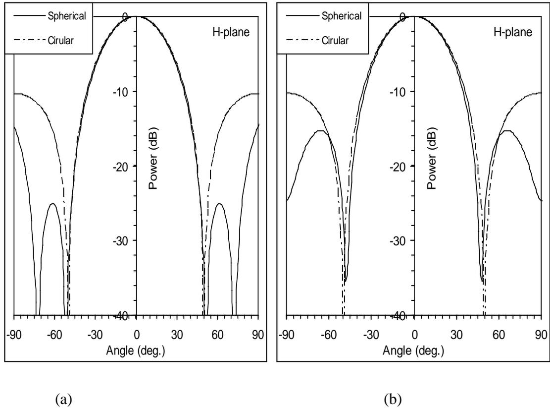
**Fig.( 4) : Radiation patterns of a uniform spherical and circular arrays a point source elements with  $R = \lambda / 2$  (a) (Spherical ( $N_0 = 4, N_{\pm 1} = 2$ ),Circular ( $N = 8$ )), (b) (Spherical ( $N_0 = 5, N_{\pm 1} = 2$ )Nm=5X2 ,Circular ( $N = 9$ ))**
