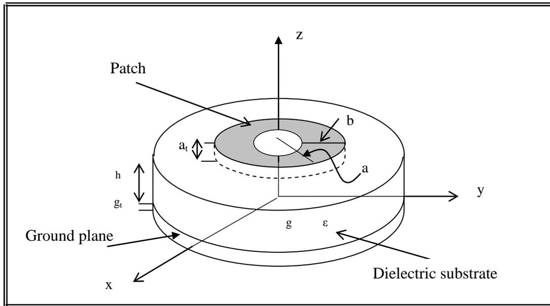
**Fig.(3) : Geometry of the annular ring microstrip antenna .**
