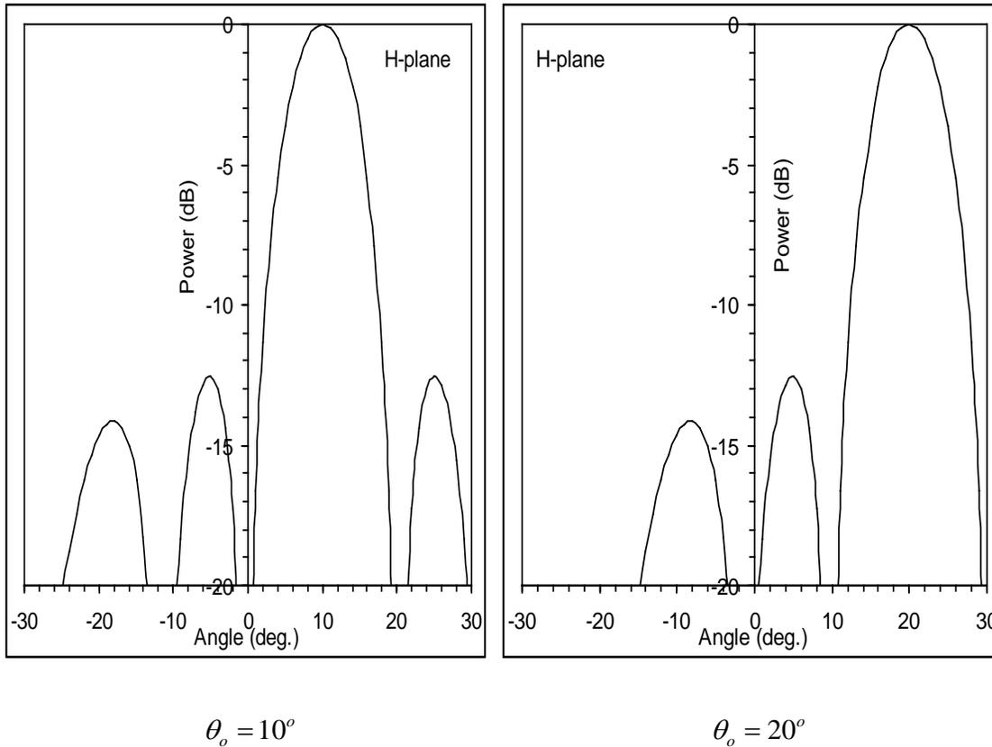
**Fig.(10) : Radiation patterns of a uniform spherical array for different elements phase.**
