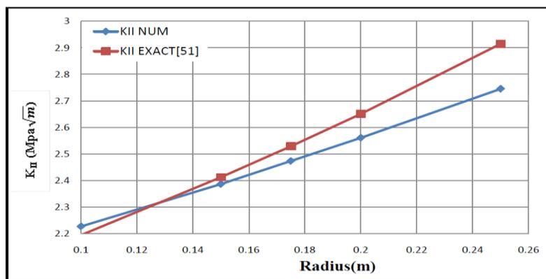
Fig. 15 Comparison of  $K_{II}$  values with exact solutions for different crack blunt radii.
