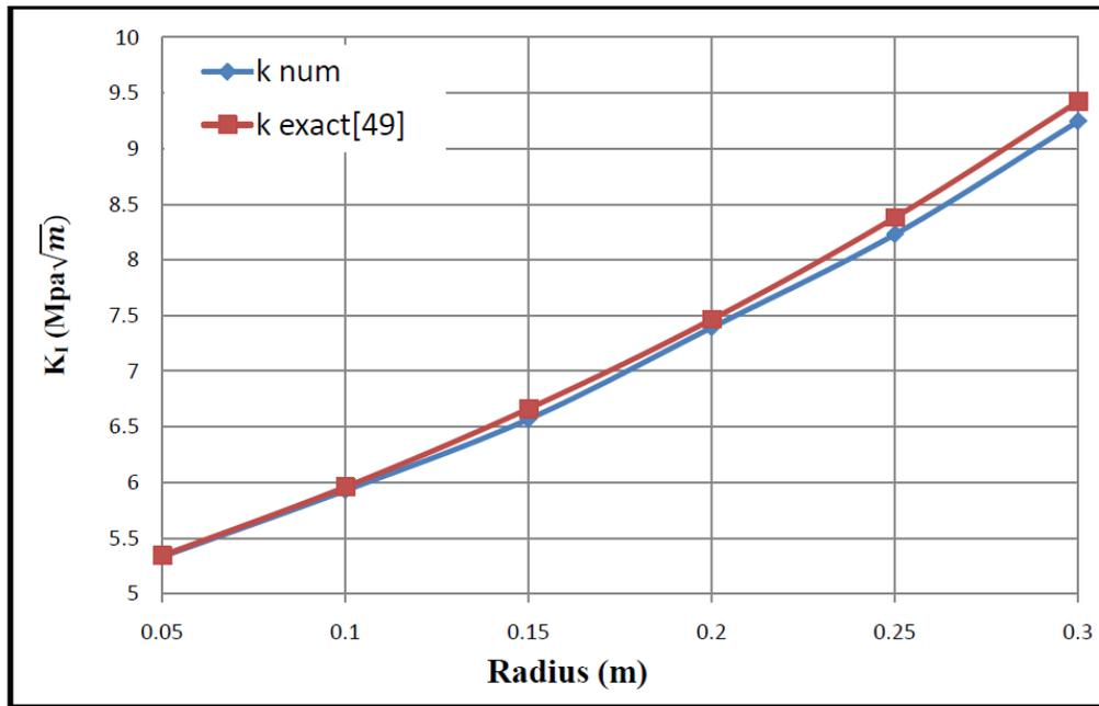
Fig. 6 Comparison of  $K_I$  values with exact solutions for different crack tip blunting.
