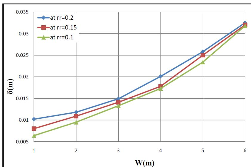
Fig.11 Crack opening displacement for different plate width at three blunt radii.
