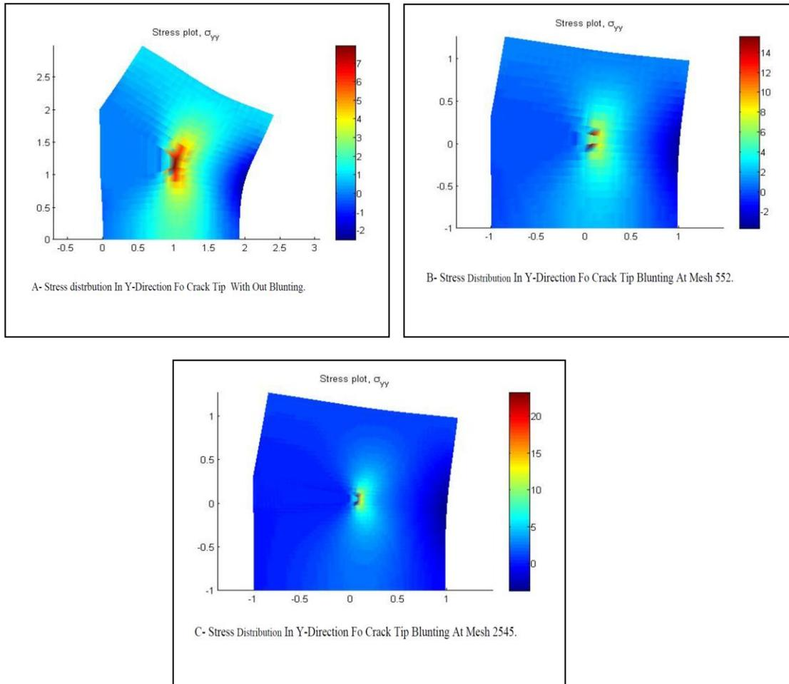
**Fig. (12)** The behavior of singularity at the crack tip in the y-direction with and without Crack tip blunting.
