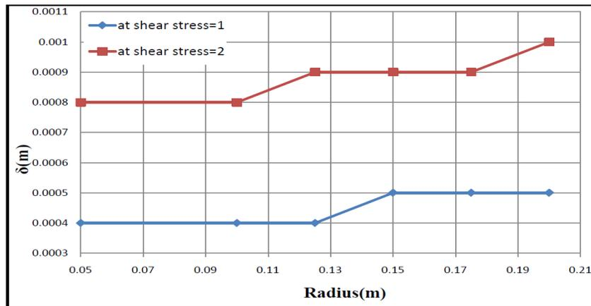
**Fig. 17** Crack opening displacement for different crack blunting radii for two shear stress values.
