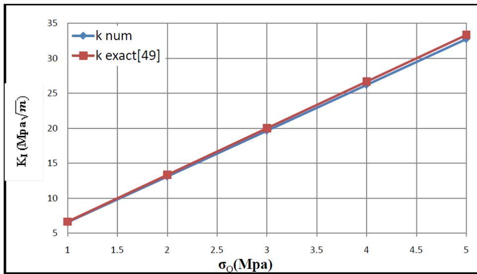
Fig. 7 Comparison of  $K_I$  values with exact solutions for different applied stresses.
