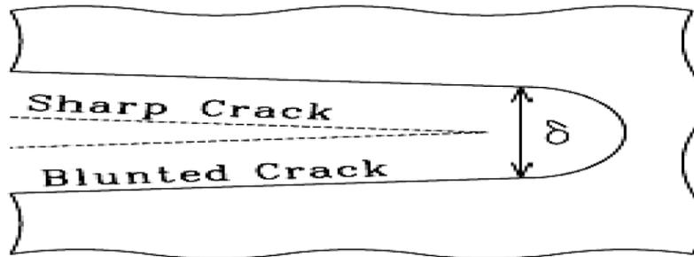
**Fig.1 Crack tip opening displacement at blunted crack [17].**
