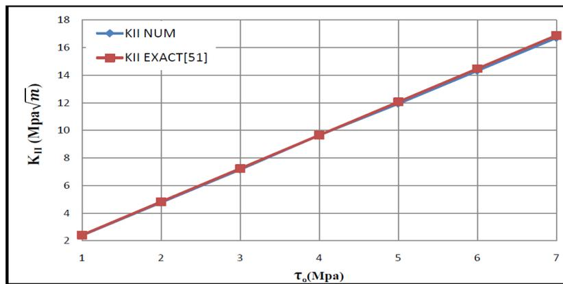
Fig. 14 Comparison of  $K_{II}$  values with exact solutions for different shear stress values.
