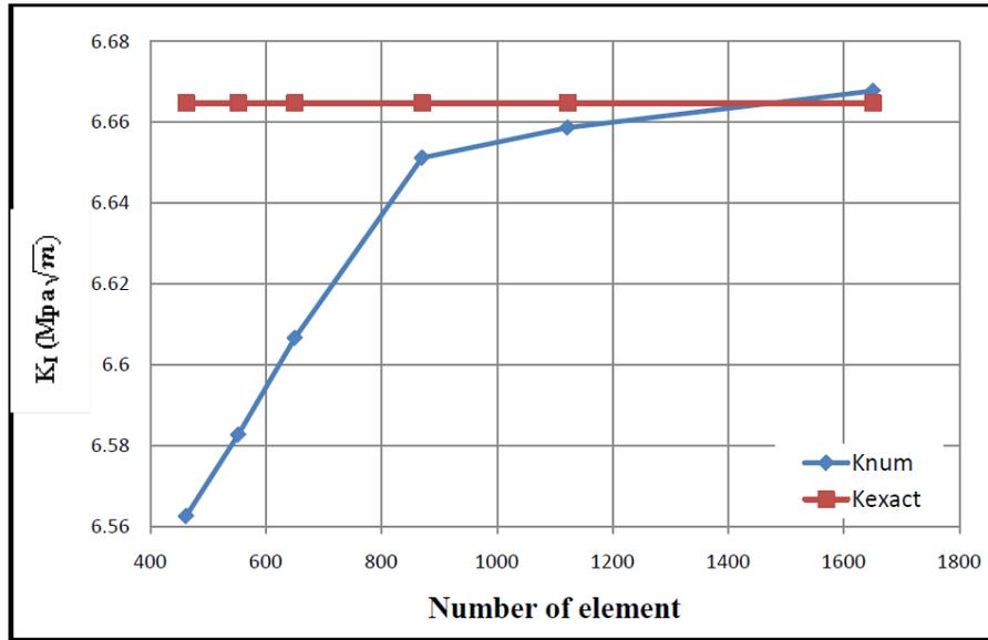
Fig. 8 Comparison of  $K_I$  values with exact solutions for different number of elements.
