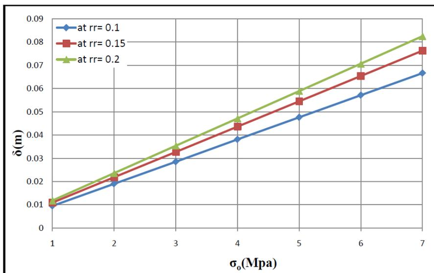
Fig. 10 Crack opening displacement for different applied stress at three blunt radii.
