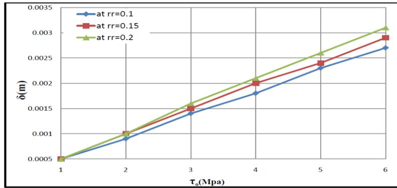
**Fig. 16** Crack opening displacement for different applied shear stress for three radii of crack blunting.
