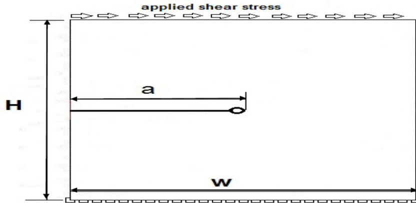
Fig. 13 An edge crack with blunted tip under shear stress.
