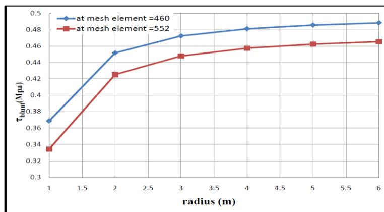
**Fig. 18** Blunting Shear stress for Mode II at different radii from the crack tip.
