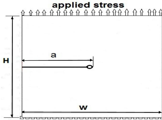
**Fig.4** An edge crack with blunted tip under tensile stress.
