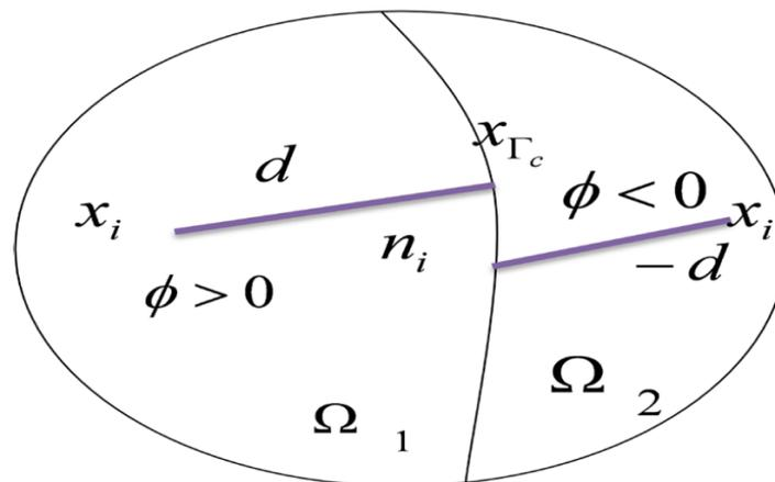
Fig.3 Definition of Signed distance function on discontinuous domain.
