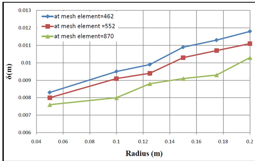
Fig. 9 Crack opening displacement for different Blunt radius at three mesh sizes.
