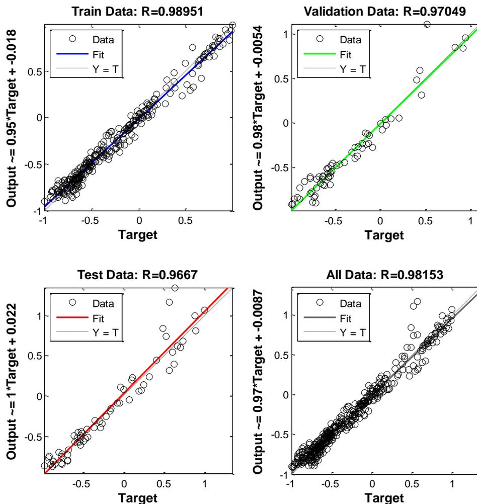
Fig. 4. Output of 6-10-1 structure model for SFC using Levenberg-Marquardt training algorithm
