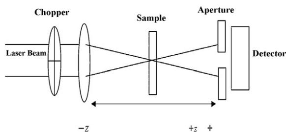
**Fig. 3.** The basic Z-scan setup.
