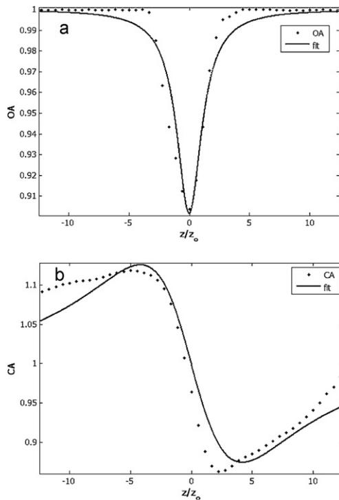
**Fig. 6.** Represent Z-scan experimental data (square) for PDPAlQ<sub>3</sub> solution: (a) open aperture and (b) close aperture, solid line shows theoretical fit to the experimental data.
