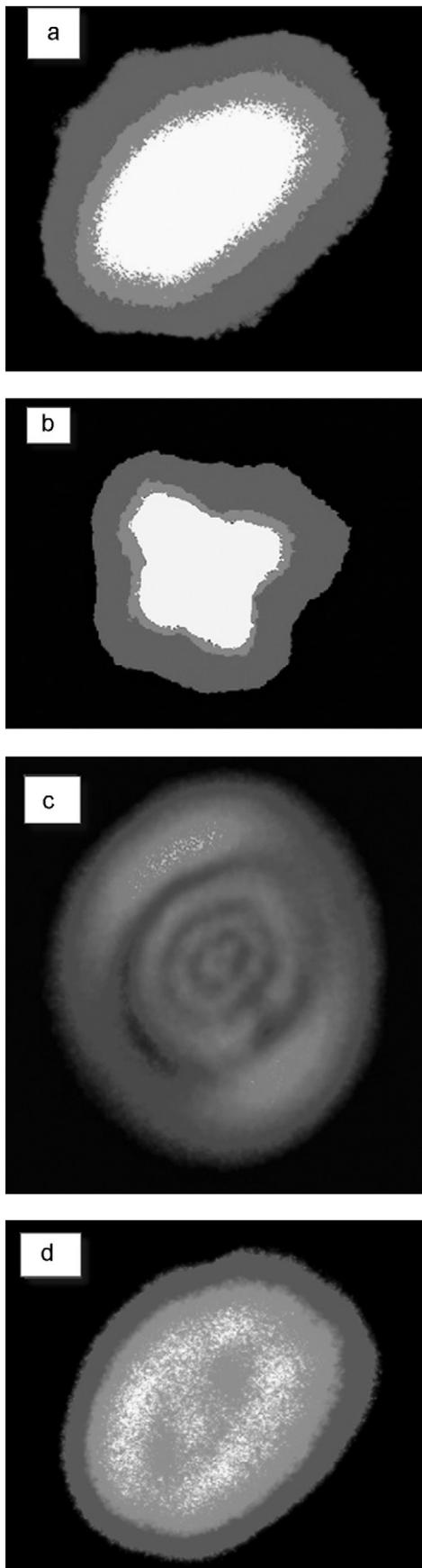
**Fig. 4.** The transmitted beam profiles corresponding to the sample positions: (a) far from the focus, (b) at the focus, (c) out of focus and (d) away from the focus for PDPAlq<sub>3</sub> solution.
