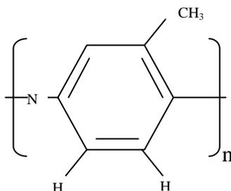
Fig.1 : structure of POT
