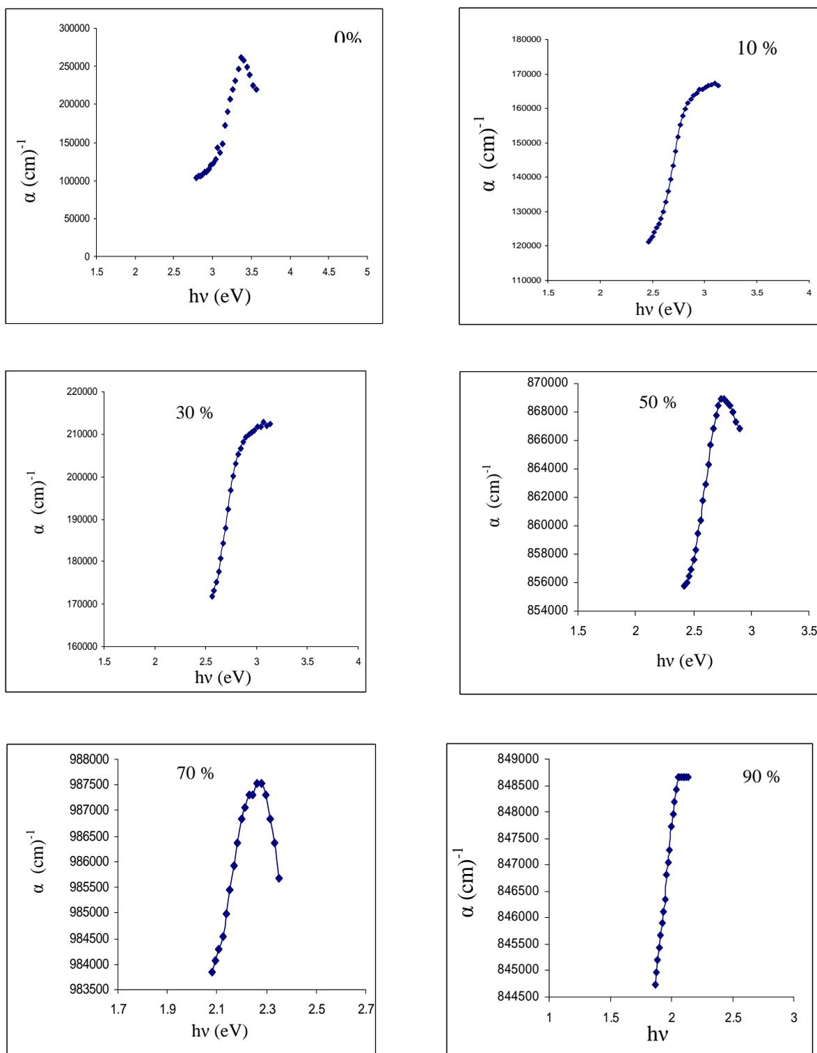
FIG.3 the absorption coefficient  $\alpha$  as a function of photon energy for different ratio of POT in POT/PEO alloys film
