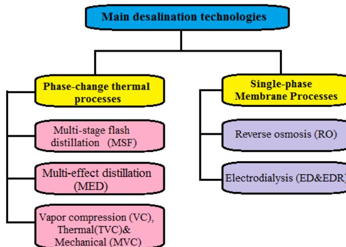
Figure 2: Desalination technologies.
