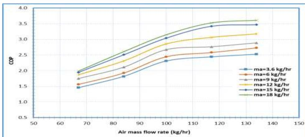
Figure10: Effect of mass flow rate of air on the (COP) at different mass flow rate of the feed water (OAOW)
