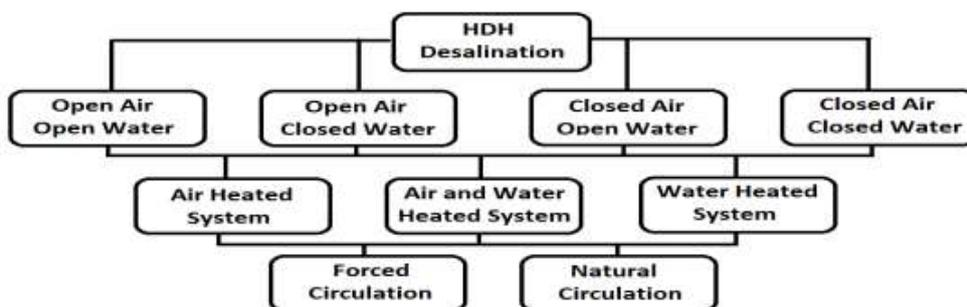
Figure 3: Classifications of HDH desalination [14]
