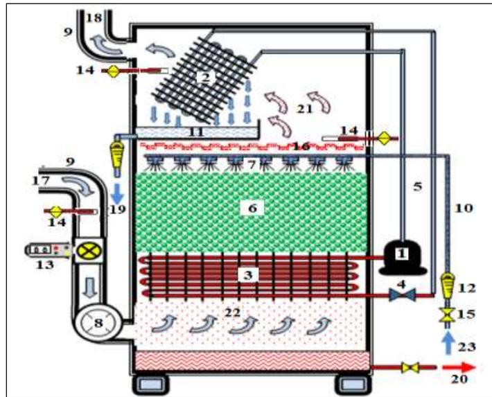
Figure 4. illustrates a schematic of the desalination unit. (1-Compressor, 2-Evaporator, 3-Condenser 4-Capillary tube, 5-Heat pump pipes, 6-Packing material, 7-Water distributor, 8-Air blower, 9- Air duct, 10-Water pipes,11-Distillate collector, 12-Rotameter,13-Anemometer, 14-Thermometer and Hygrometer,15-Water valve, 16-Droplet eliminator, 17-Inlet air, 18- Out let air,19-Fresh water ,20- Brine, 2-Humid air ,22- Water droplets, 23- Feed water).
