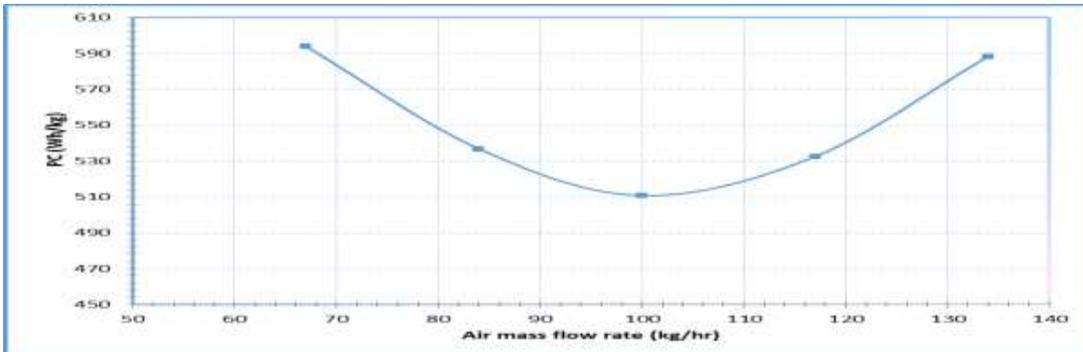
Figure 9: Effect of mass flow rate of air on the consumed power (Wh/kg) at constant mass flow rate of feed water (OAOW).
