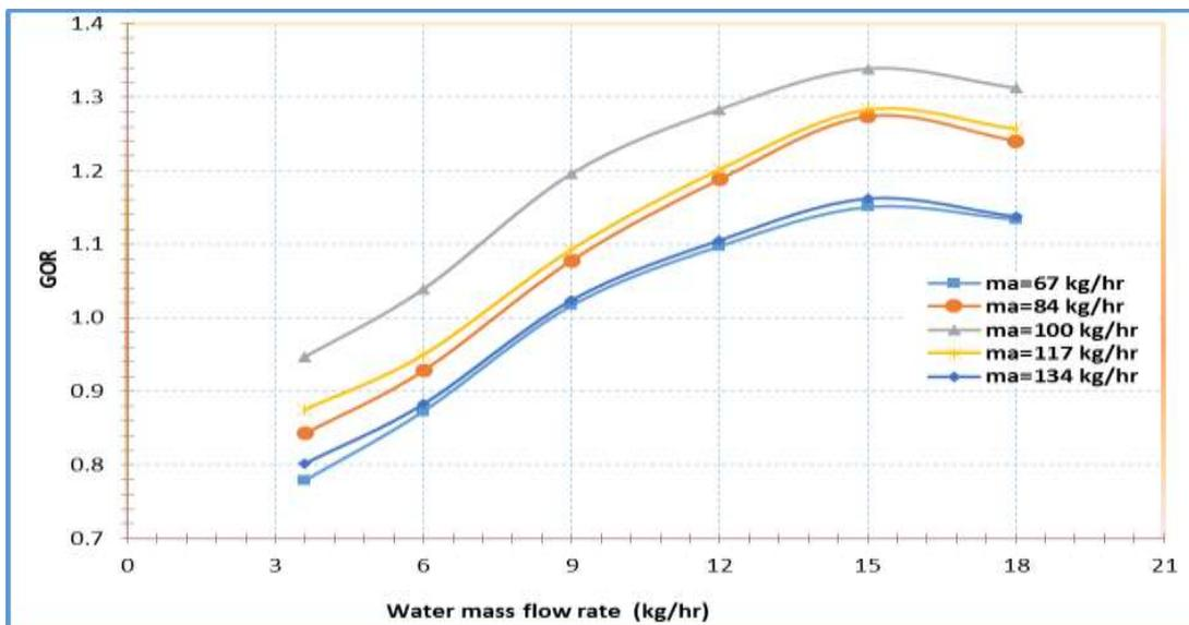
Figure 6: Effect of mass flow rate of feed water on the gained output ratio(GOR) at different mass flow rate of air (OAOW).
