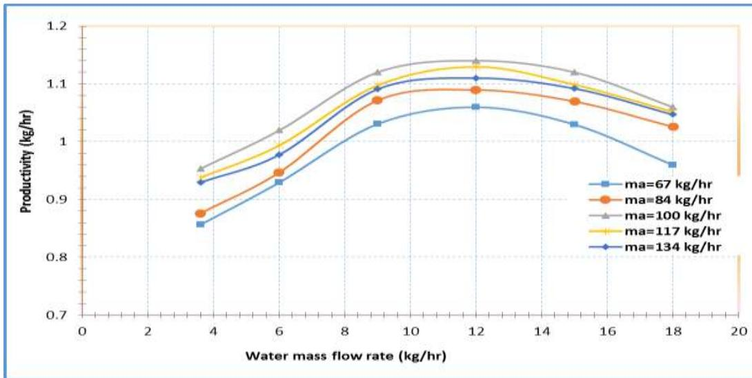
Figure 5: Effect of mass flow rate of feed water on productivity at different mass flow rate of air (OAOW).
