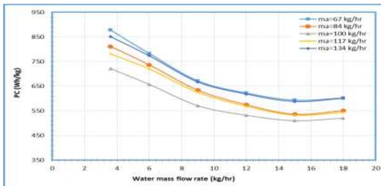
Figure 8: Effect of mass flow rate of feed water on the consumed power (Wh/kg) at different mass flow rate of air (OAOW).
