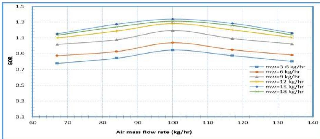
Figure 7 Effect of mass flow rate of air on the gained output ratio (GOR) at different mass flow rate of feed water (OAOW).
