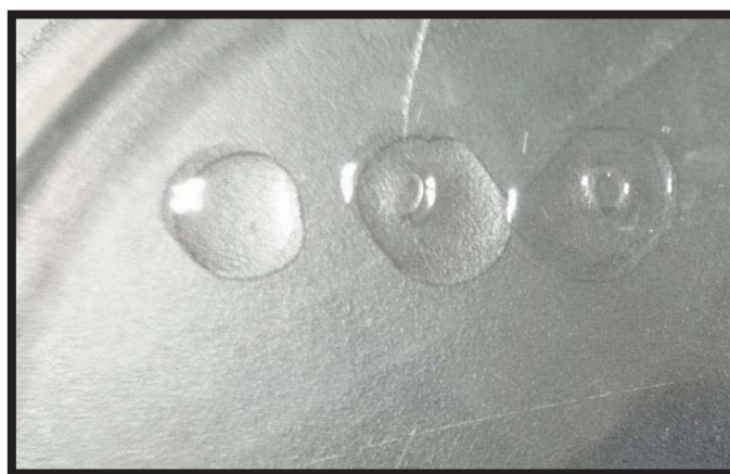
Fig. (5) Oil collapse of mineral oil drops.
