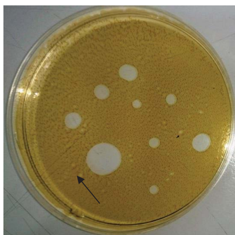
Fig. (3) Dispersion of crude oil by biosurfactant.
