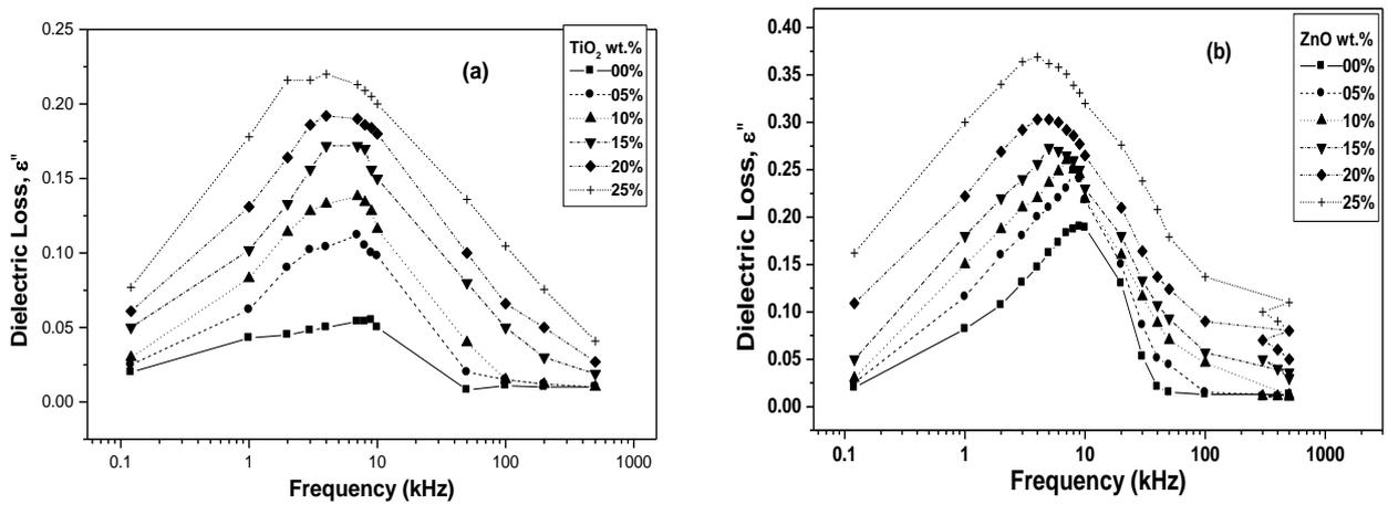
Fig. (5) Dielectric Loss as a function of filler content and frequency for different content of (a)  $TiO_2$  and (b) ZnO- epoxy composite.
