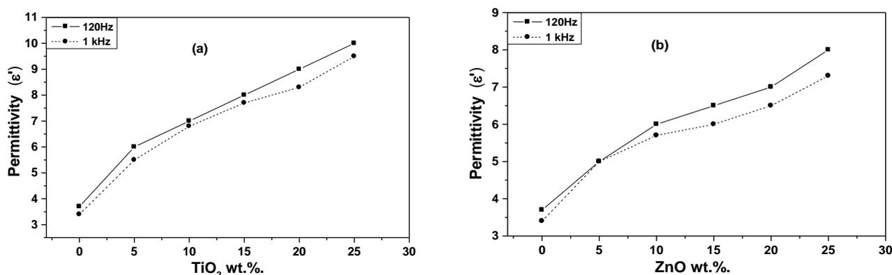
**Fig. (1).Variation of permittivity with two different frequencies (a) TiO<sub>2</sub> and (b) ZnO**
