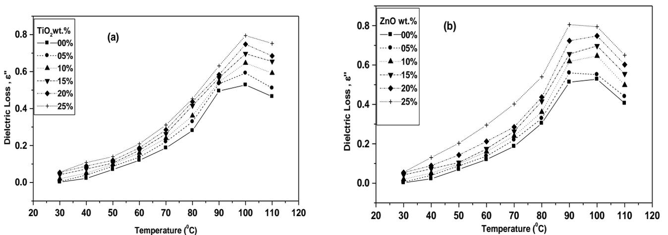
Fig. (3) Dielectric loss as a function of temperature for different content of (a) TiO<sub>2</sub> and (b) ZnO- epoxy composite.
