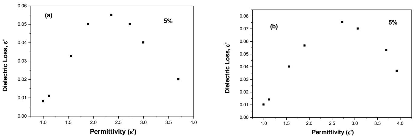
Fig. (7) Cole-Cole diagram for (a)  $TiO_2$ - epoxy composite and (b) ZnO- epoxy composite.
