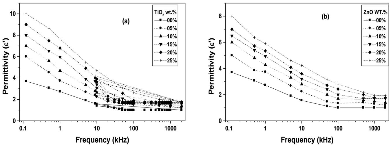
Fig. (3) The permittivity as a function frequency for different content of (a) TiO<sub>2</sub> and (b) ZnO- epoxy composite.
