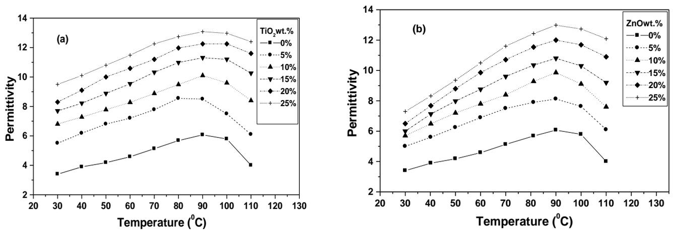
Fig. (2) Permittivity as a function of temperature for different content of (a) TiO<sub>2</sub> and (b) ZnO- epoxy composite.
