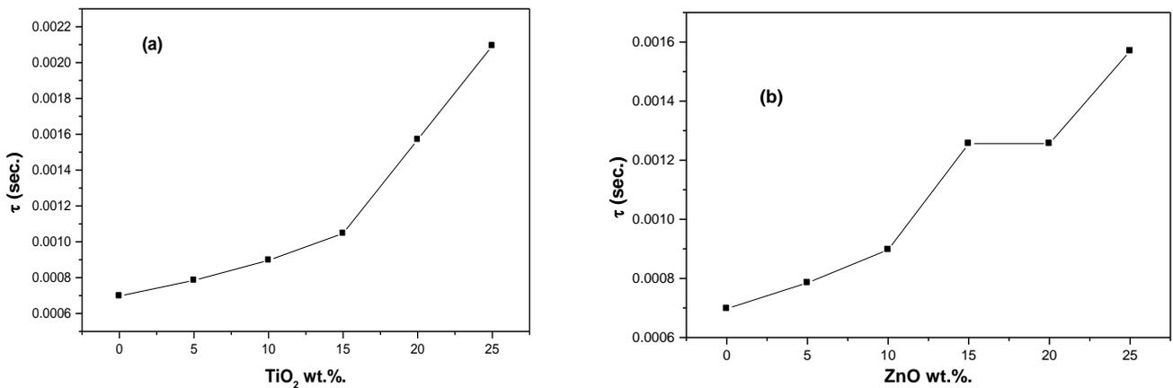
Fig. (6) Relaxation time as a function of filler content for (a)  $TiO_2$  and (b) ZnO- epoxy composite.
