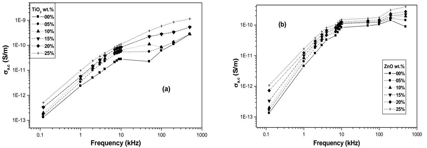
Fig.(9) AC conductivity as a function of frequency for different content of (a) TiO<sub>2</sub> and (b) ZnO- epoxy composite.
