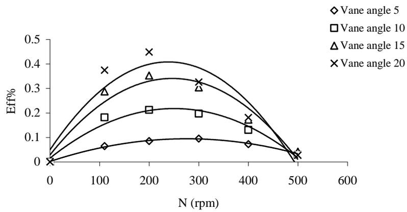
Fig. 6. Turbine efficiency versus shaft speed
