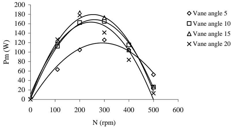
Fig. 4. Turbine mechanical power versus shaft speed
