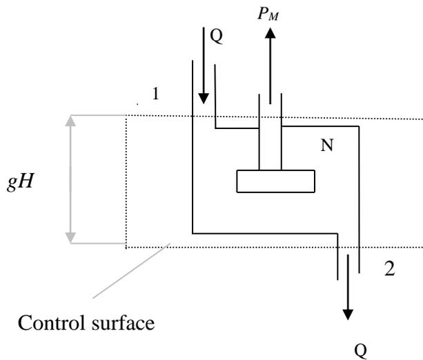
Fig.1. Cross flow turbine control volume
