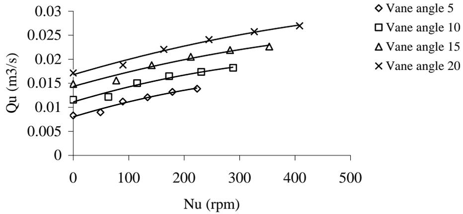
Fig. 8. unit flow versus unit speed
