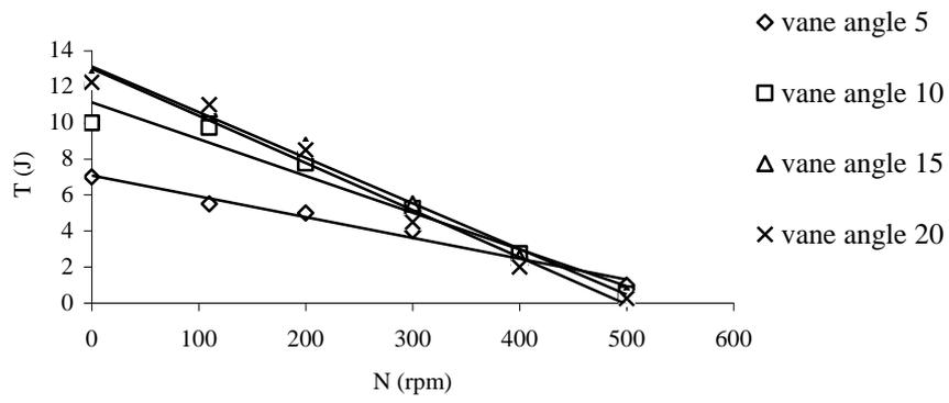
Fig. 5. Torque versus shaft speed
