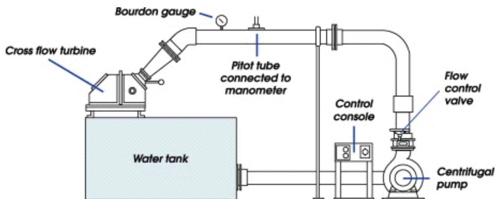
Fig. 2. Schematic of circuit ( brake and tachometer omitted for clarity) [4].
