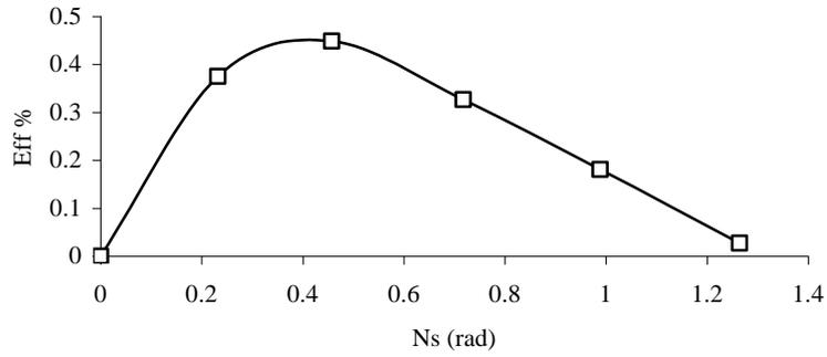
Fig. 9. Turbine efficiency versus dimensionless specific speed
