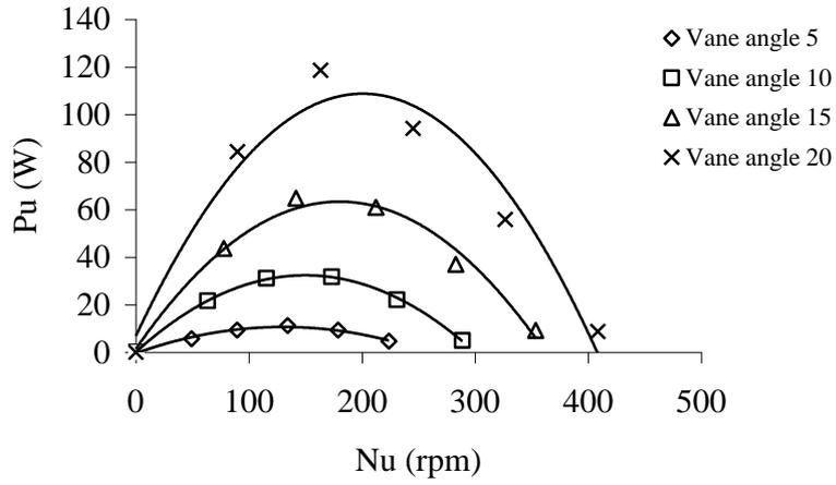
Fig. 7. Unit power versus unit speed
