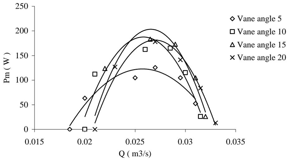
Fig. 3. Turbine mechanical power versus input water flowrate
