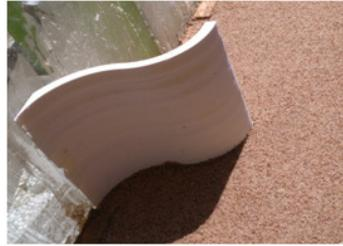
**Plate 2** The S-shape groyne placed in the flume
