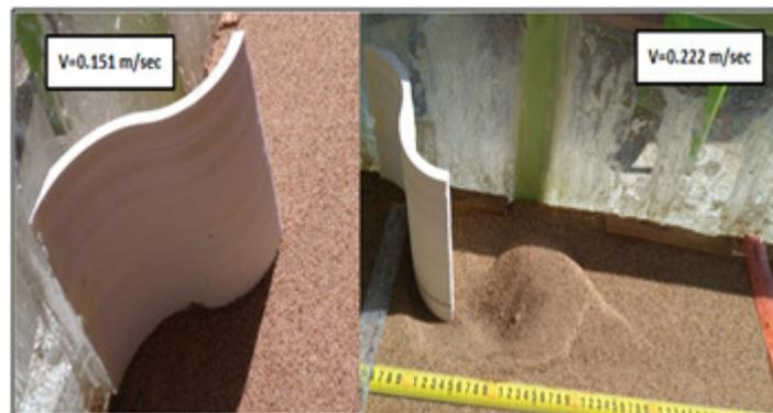
**Plate 4** Effect of flow velocity on scour depth development
