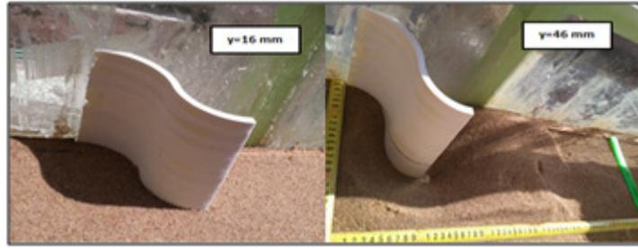
**Plate 3** Effect of flow depth on scour depth development
