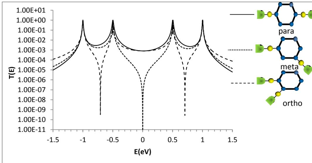
**Fig.(2): the transmission probability as function of the system energy with  $E_{B1}= E_{B2}=E_{B3}= E_{B4}= E_{B5}= E_{B6}=0$ ,  $V^{DB}=V^{AB}=-0.3eV$ ,  $V^{BB}=-0.5eV$ ,  $V^{AR}=-3eV$ ,  $\beta_R=-3eV$ ,  $\phi=0$ .**
