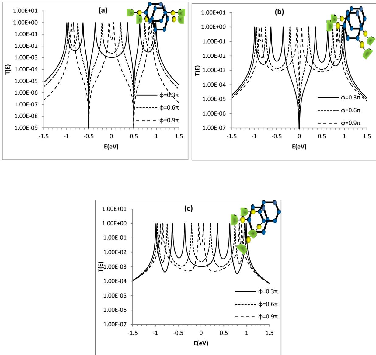
**Fig.(3):** The transmission probability as function of the system energy with presence magnetic flux at  $\phi = 0.3\pi, 0.6\pi, 0.9\pi$  for three configurations are para in (a), meta in (b) and ortho in (c). The parameters are  $E_{B1} = E_{B2} = E_{B3} = E_{B4} = E_{B5} = E_{B6} = 0$ ,  $V^{DB} = V^{AB} = -0.3\text{eV}$ ,  $V^{BB} = -0.5\text{eV}$ ,  $V^{AR} = -3\text{eV}$ ,  $\beta_R = -3\text{eV}$ .
