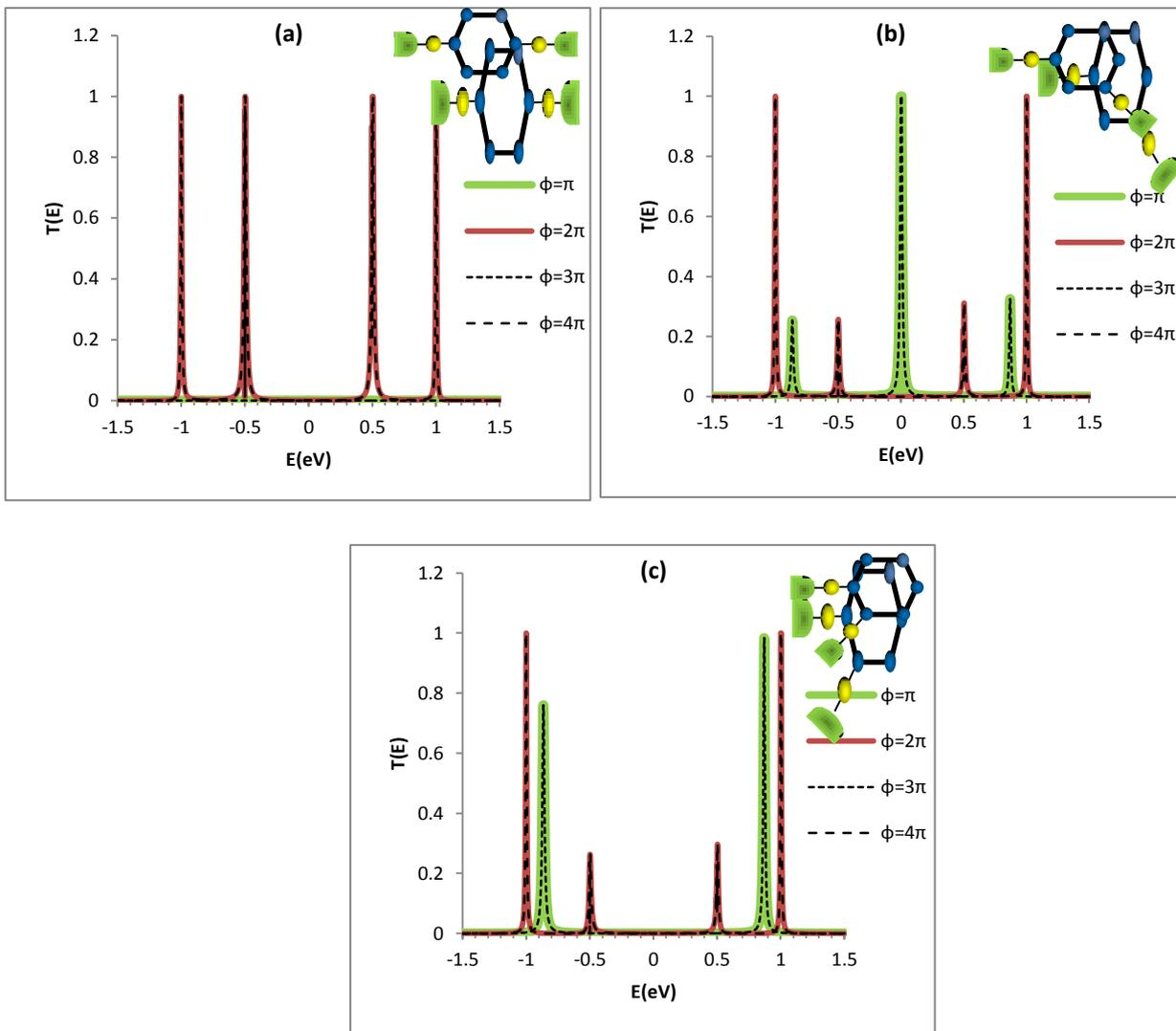
Fig.(4): The transmission probability as function of the system energy with presence magnetic flux at  $\phi = \pi, 2\pi, 3\pi, 4\pi$  for three configurations are para in (a), meta in (b) and ortho in (c). The parameters are  $E_{B1}=E_{B2}=E_{B3}=E_{B4}=E_{B5}=E_{B6}=0$ ,  $V^{DB}=V^{AB}=-0.3\text{eV}$ ,  $V^{BB}=-0.5\text{eV}$ ,  $V^{AR}=-3\text{eV}$ ,  $\beta_R=-3\text{eV}$ .
