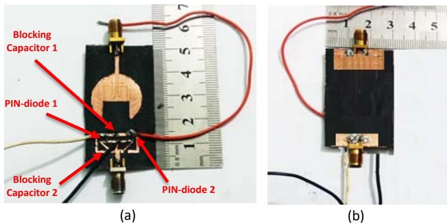
Figure 10: Prototype of the proposed antenna system (a) front view (b) back view.
