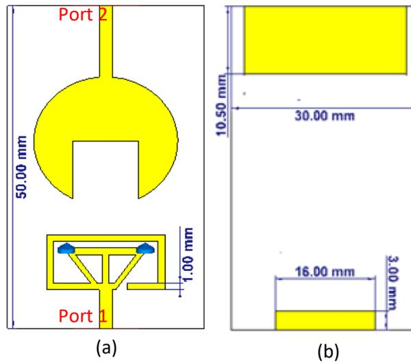
Figure 1: Structure of the proposed antenna system (a) front view, (b) back view
