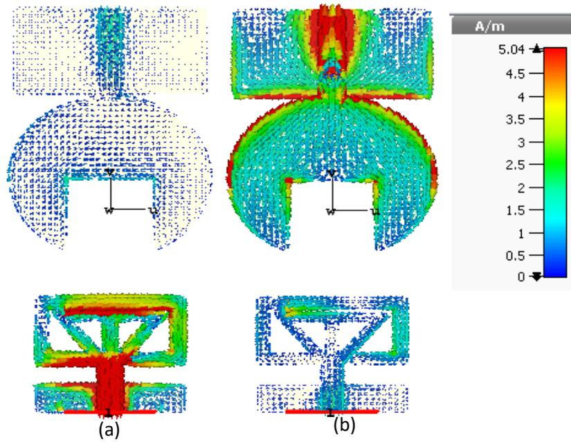
Figure 9: Current distribution of the propose antenna system at  $f=5\text{GHz}$ , and PIN diode -1 ON PIN diode-2 OFF when (a) port 1 is excited and (b) port 2 is excited.
