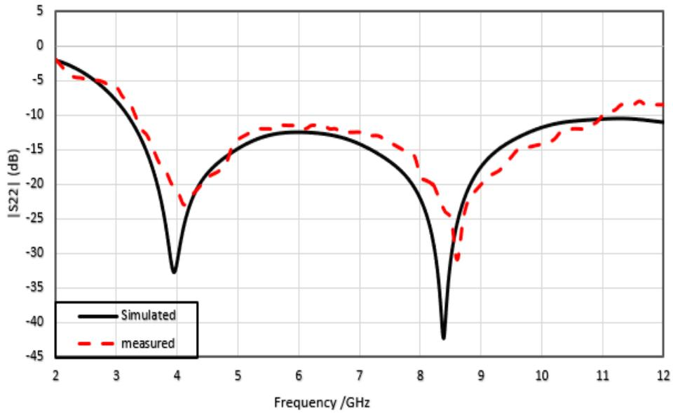
Figure 11: Simulated and measured reflection coefficient of the UWB sensing antenna.
