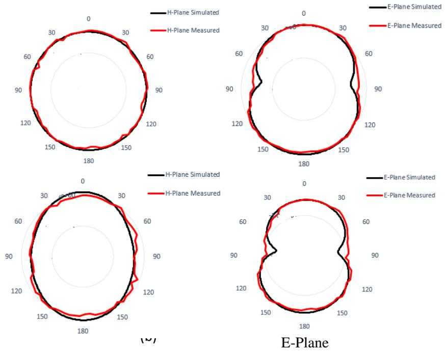
Figure 12: Simulated and measured power patterns (a) E and H plane for 4GHz (b) E and H plane for 8.4GHz
