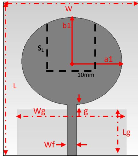
Figure 4: Structure of the elliptical monopole sensing antenna.
