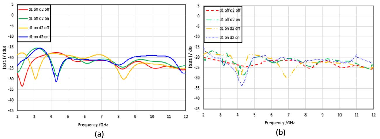
Figure 16: Forward transmission coefficient of the proposed antenna system for different PIN diode states (a) simulated and (b) measured.
