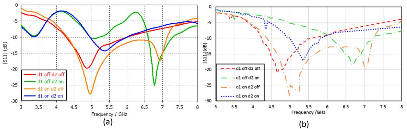
Figure 14: Reflection coefficients of the communicating antenna for different PIN diodes states (a) simulated and (b) measured.
