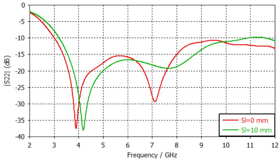
Figure 8: Comparison of the reflection coefficient of the sensing antenna with and without the slot.
