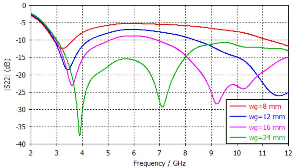
Figure 6: Reflection coefficient of the sensing antenna for  $a_1=11\text{mm}$ ,  $b_1=10\text{mm}$ , and different value of ground plane width.
