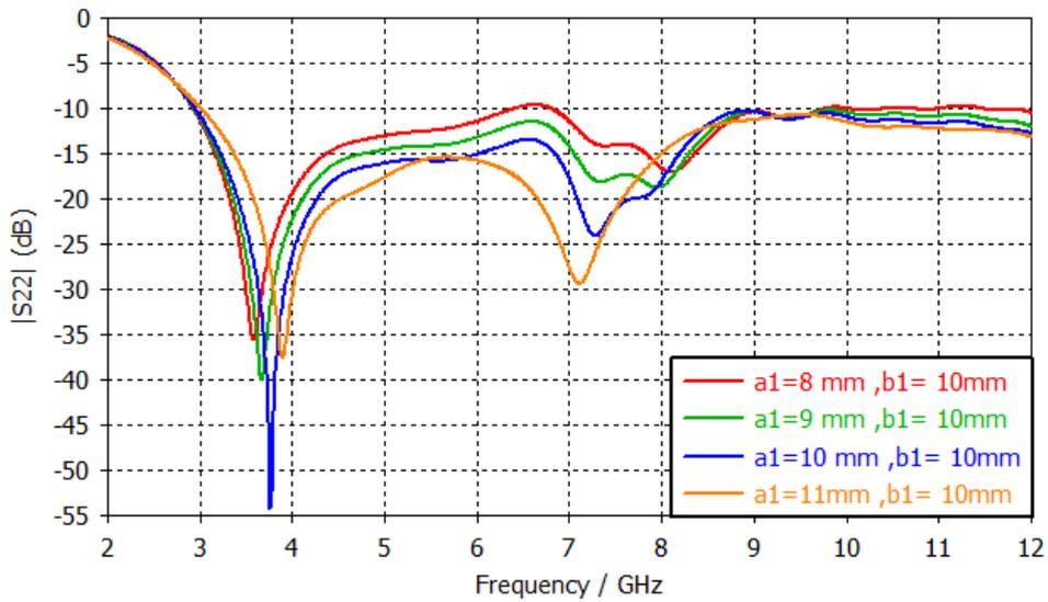
Figure 5: Reflection coefficient of the sensing antenna for  $w_g=24\text{mm}$  and different value axial ratio.
