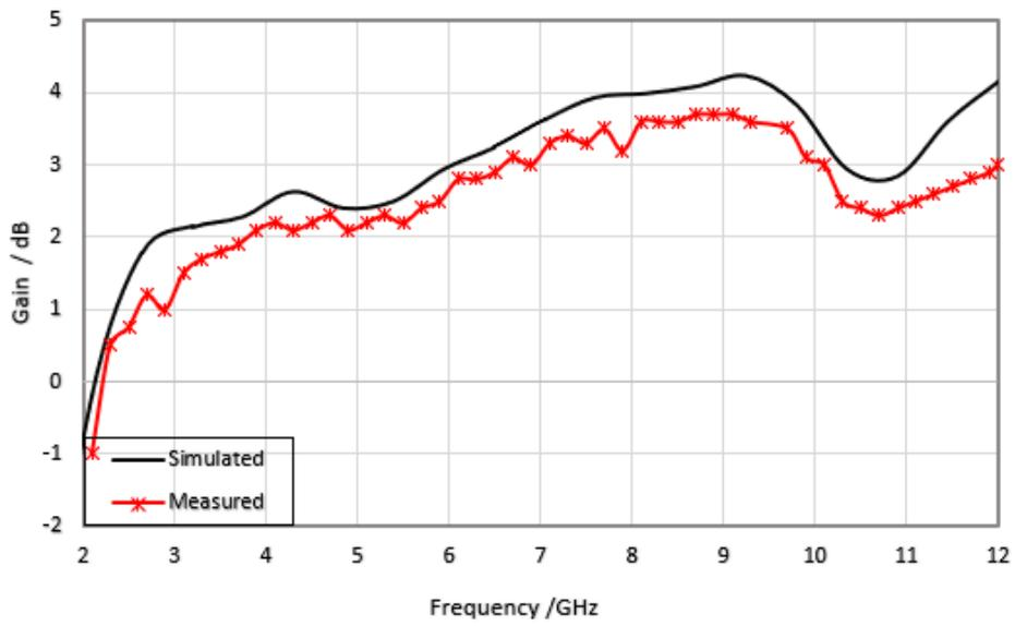
Figure 13: Simulated and measured gain for proposed sensing antenna.
