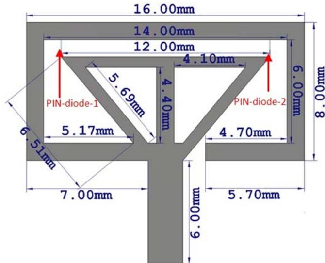
Figure 2: Structure of the reconfigurable communicating antenna.
