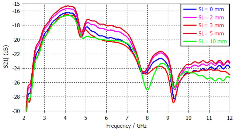
Figure 7: Mutual coupling of the proposed antenna system for different value of slot length.
