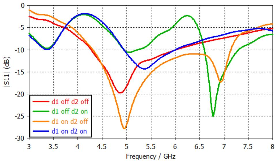
Figure 3: Simulated reflection coefficients for different PIN diodes states.
