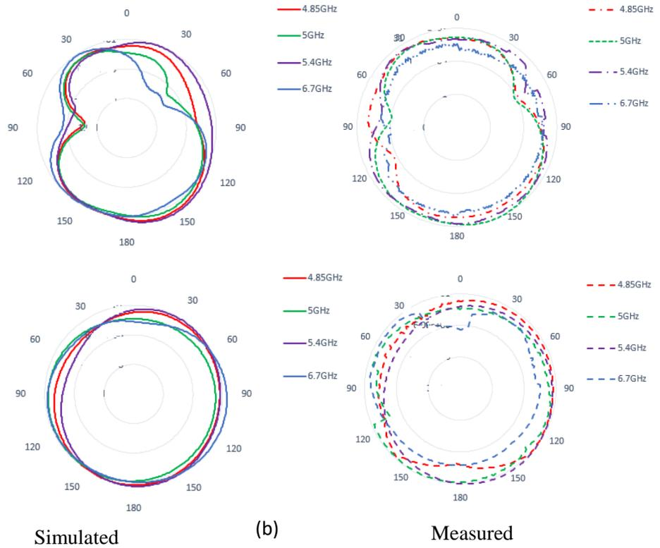
Figure 15: Simulated and measured power patterns of the communicating antenna for different PIN diode states (a) E-PLANE (b) H-PLANE
