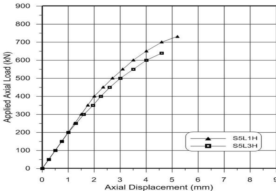
**Figure 13: Effect of the Slenderness Ratio on the Behavior Tested Square HSCFDST Column Specimens**
