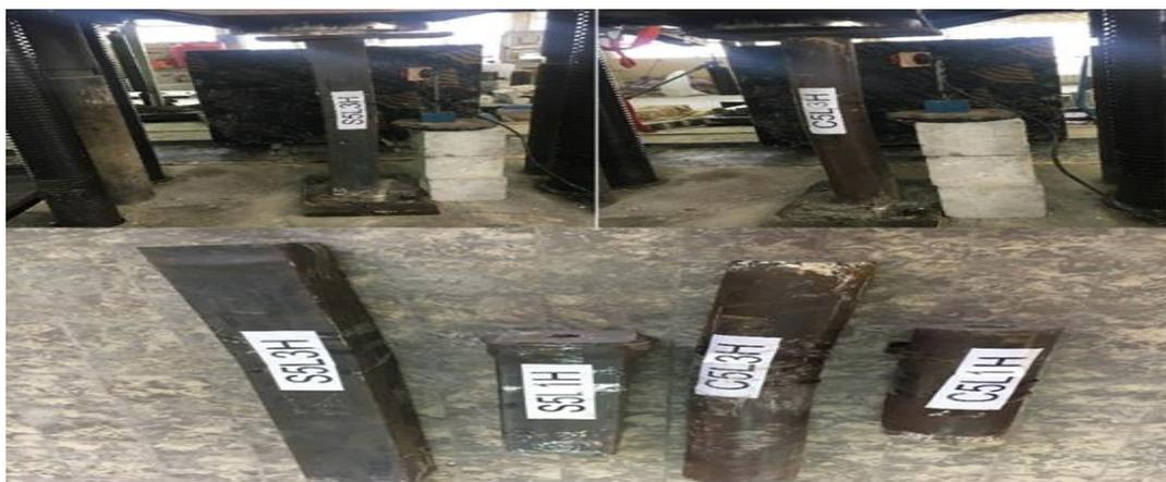
Figure 6: Mode of Failure for Specimens C5L3H and S5L3H
