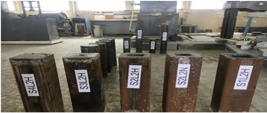
**Figure 3: Preparation of Tested CFDST Column Specimens**
