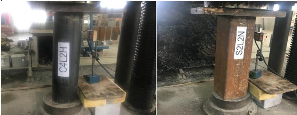
**Figure 4: Column Specimens Test Setup**
