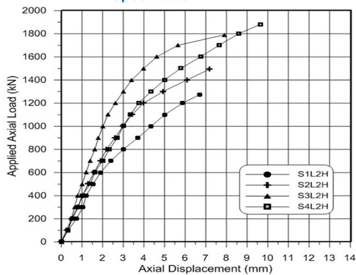
**Figure 8: Applied Axial Load - Axial Displacement Relationships for Tested HSCFDST Square Specimens**
