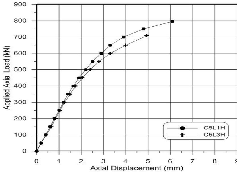
**Figure 12: Effect of the Slenderness Ratio on the Behavior Tested Circular HSCFDST Column Specimens**
