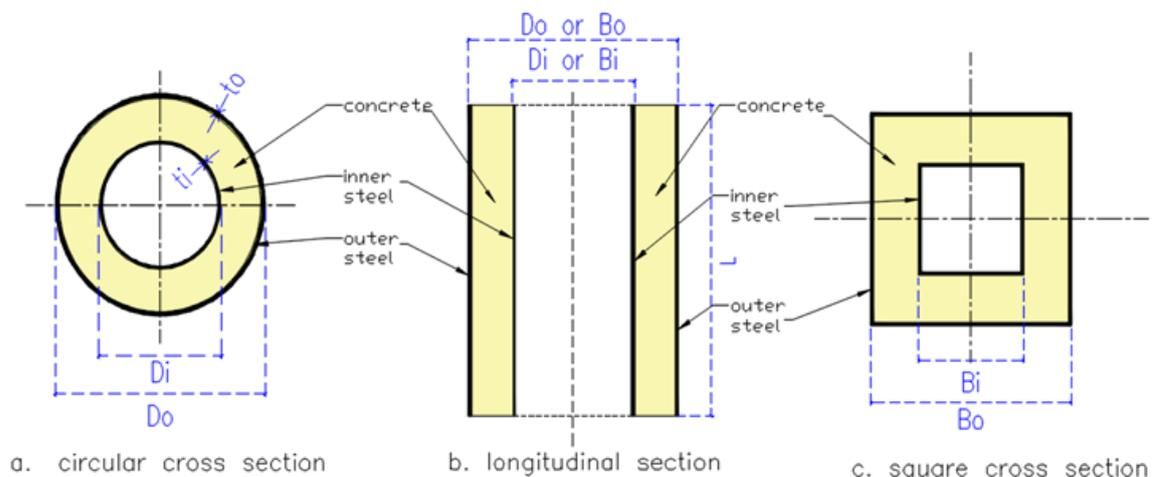
Figure 2: Details of Tested CFDST column specimens
