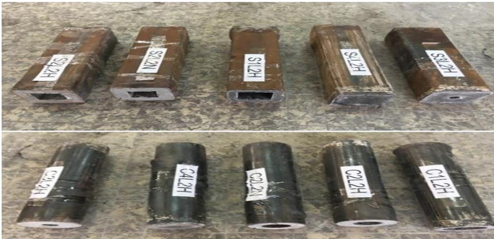
Figure 5: Mode of Failure for All Specimens Except (C5L3H and S5L3H)
