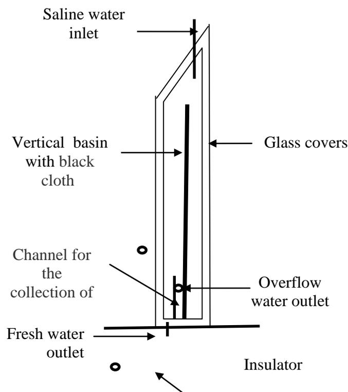
**Fig. (1) A schematic diagram of the Vertical Solar Still (VSS)**
