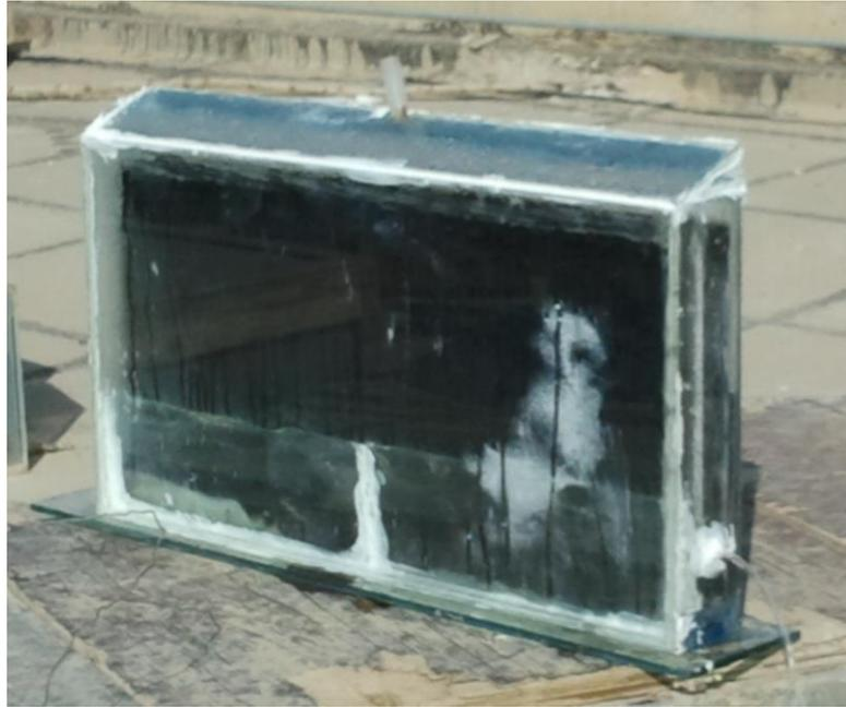
Fig.(2) A photographic picture of the Vertical Solar Still (VSS)
