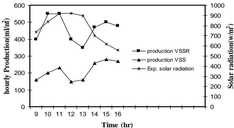
Fig. (6) Experimental hourly productivity of VSSR and VSS and the solar radiation intensity at 16 July 2012.
