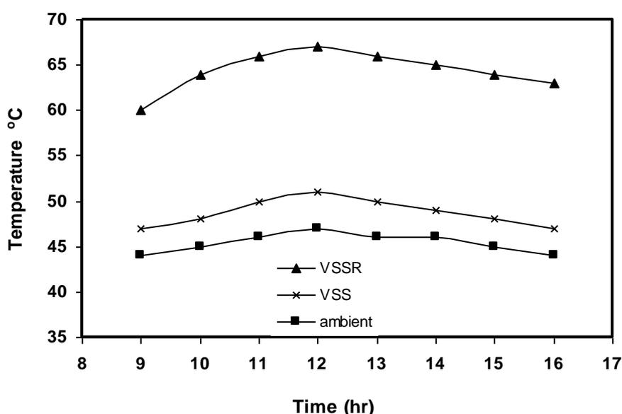
Fig. (7): The change in the temperature of the water basin along the daily hours at 16 July 2012.
