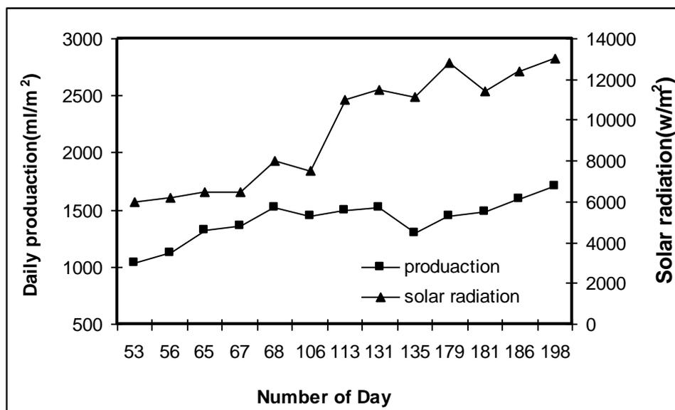
Fig. (4) Daily production of the solar still with the solar radiation from days of February to July 2012.
