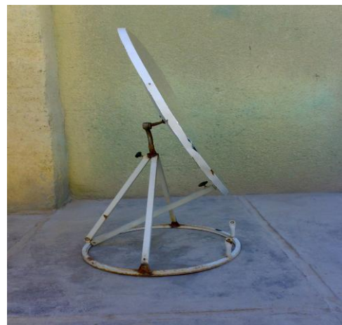
Fig. 4. Schematic diagram of the dish covered with aluminum paper [10].
