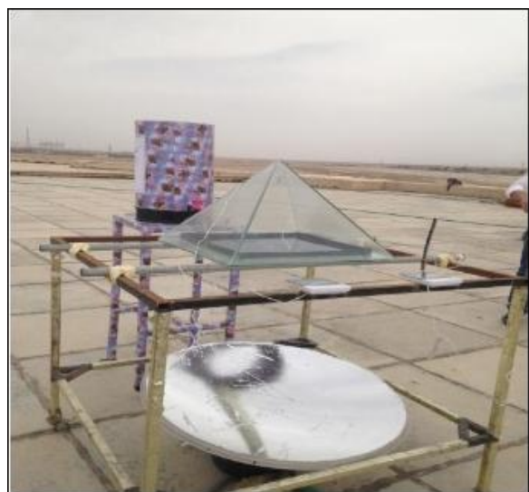
Fig. 3. Photograph picture of the pyramidal solar still (PSS) with external reflector.
