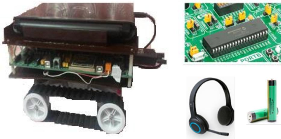
**Figure (4):** The overall designed listening robot with its main parts
