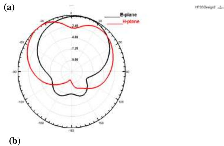
**Figure 4.** Radiation patterns for the proposed antennas with (a) coaxial probe feed (b) microstrip edge feed.
