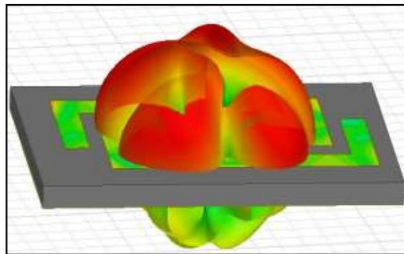
**Figure 5.** Radiation pattern in three dimensions for the proposed antennas with coaxial probe feed at resonant frequency 18.09 GHz.
