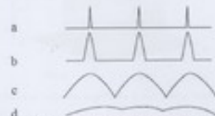
Figure 1: Distribution of pulse intensity with time at different distance. (a) Initial pulses. (b) pulses start to separate (c) starting to overlap (d) pulses no longer recognizable [3].
