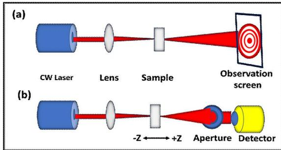
Figure 2. Experimental set-up for (a) diffraction ring patterns, (b) Z-Scan technique.
