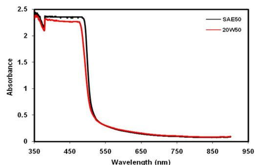
Figure 1. Linear absorbance spectrum of 20W50 and SAE 50 oils.
