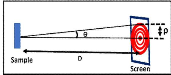
Fig.5. Definition of experimental  $\theta$ , D and  $\rho$  used in the numerical analysis of the diffraction patterns.
