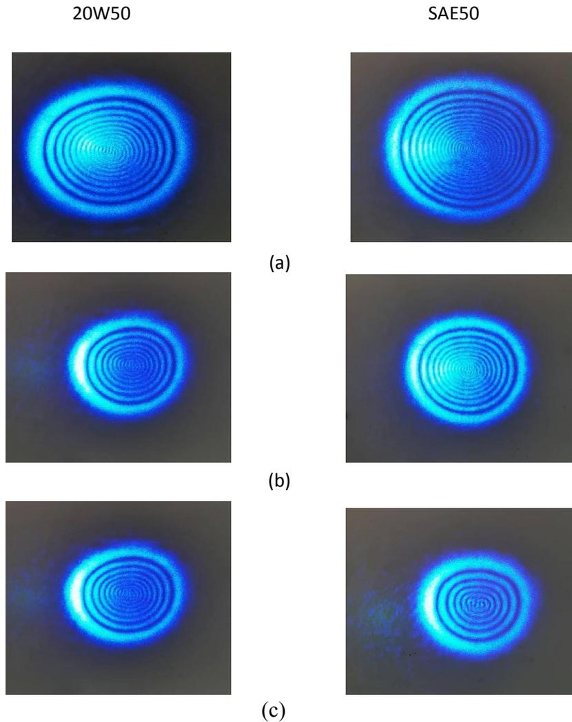
Figure (3). Diffraction ring pattern in 20W50 (left column) and SAE 50 oils (right column) at input power of (mW): (a) 48.53, (b) 37.53 and (c) 29.12.
