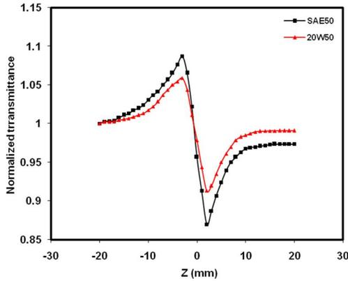
Figure 4. Closed aperture normalized Z-scan data of 20W50 and SAE 50 oils.
