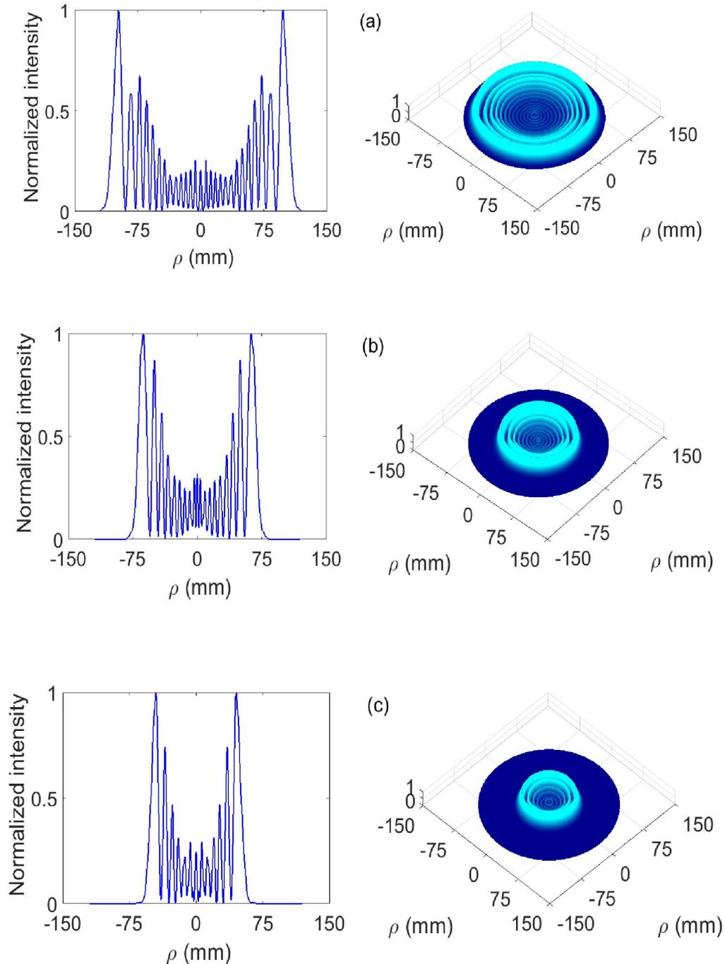
Figure (7). Intensity distribution of diffracted laser beam from SAE 50 oil at powers (mW): (a) 48.53, b) 37.53 and (c) 29.12, left and right columns are 2D and 3D distributions respectively.
