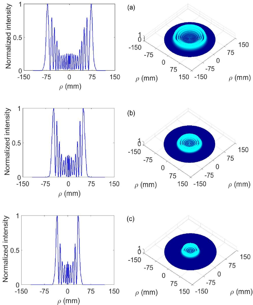
Figure (6). Intensity distribution of diffracted laser beam from 20W50 oil at powers (mW): (a) 48.53, (b) 37.53 and (c) 29.12, left and right columns are 2D and 3D distributions respectively.
