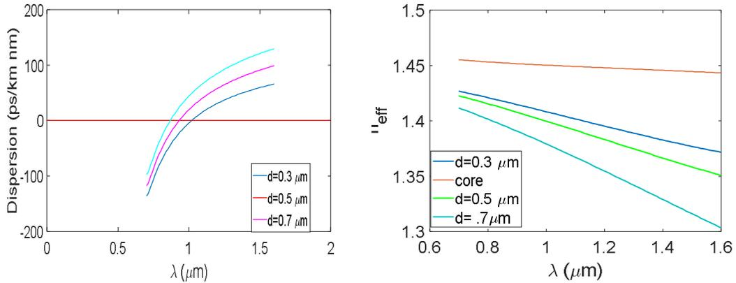
Figure (2): The dispersion curve and  $n_{eff}$  for different values of hole diameter.
