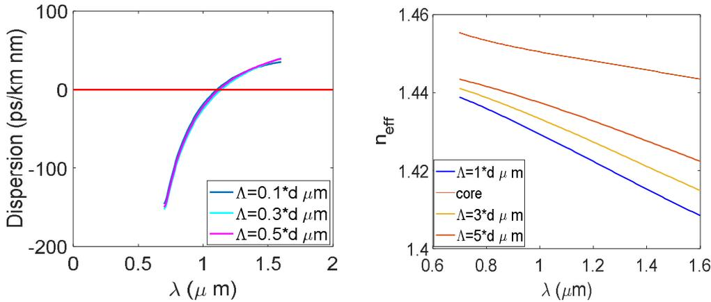
Figure (1): The dispersion curves (left), and  $n_{eff}$ (right), changes with wavelength at  $d=0.3 \mu m$ ,  $N=5$ .
