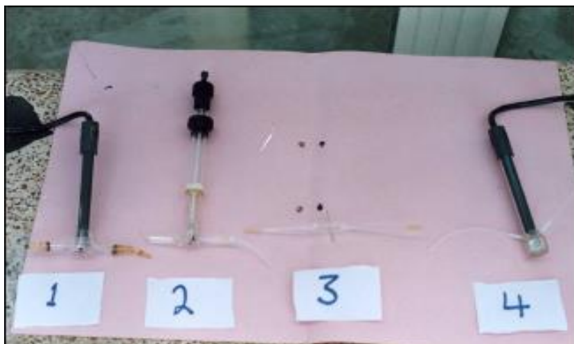
Fig.2 The four home-made flow cells which designed in our laboratory
