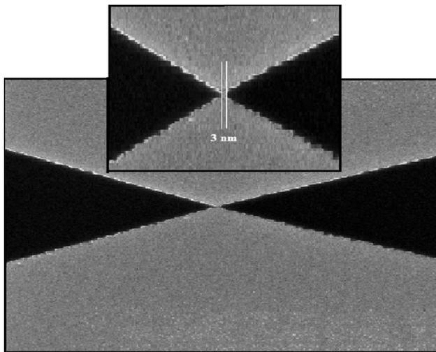
**Fig. 2** FESEM images show 3 nm gold electrode pattern after using an aqua regia solution (HCl 1:3 HN<sub>3</sub>) sequent to remove undesired gold material between the two electrodes
