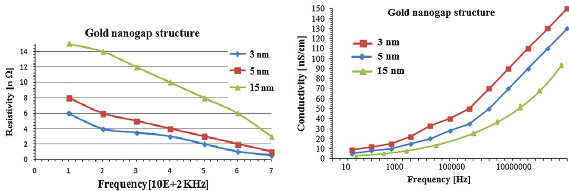
**Fig. 3** Resistivity and conductivity parameters for the gold devices with different nanogaps size
