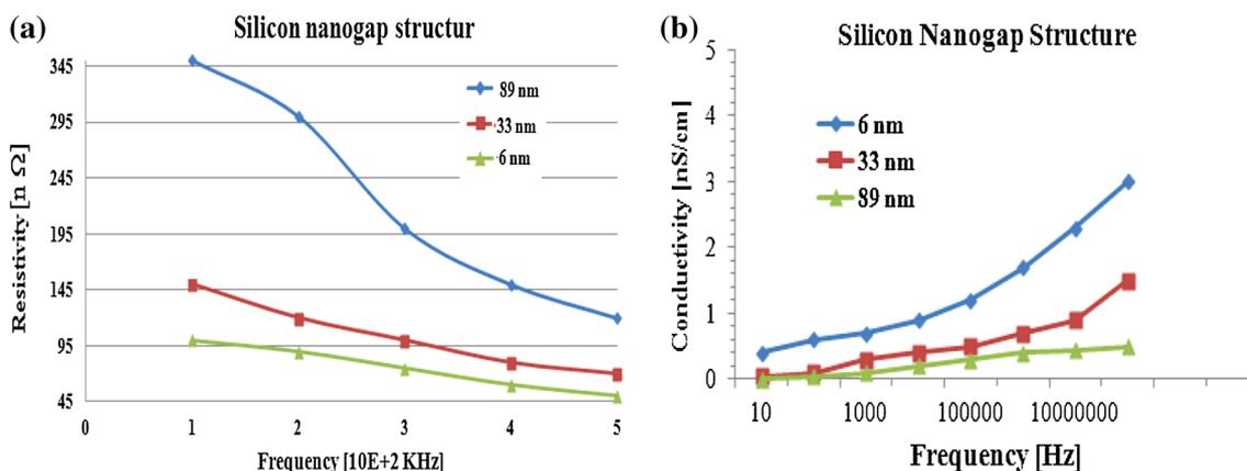
**Fig. 7** Resistivity and conductivity parameters for the silicon devices with different nanogaps size
