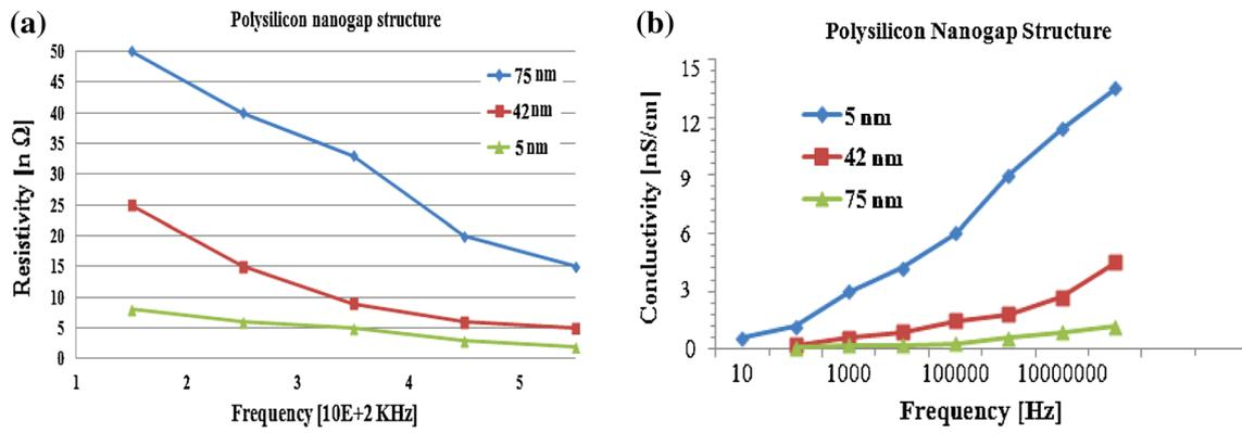
**Fig. 5** **a** resistivity and **b** conductivity parameters for the devices with different nanogaps size
