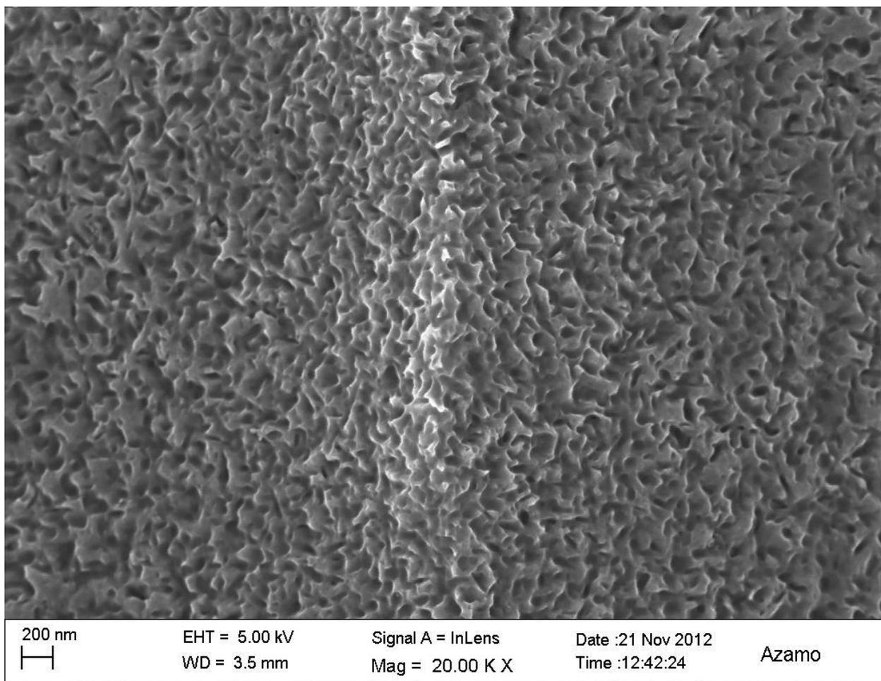
Fig1. Surface SEM micrographs of porous silicon samples fabricated ultrasonic etching
