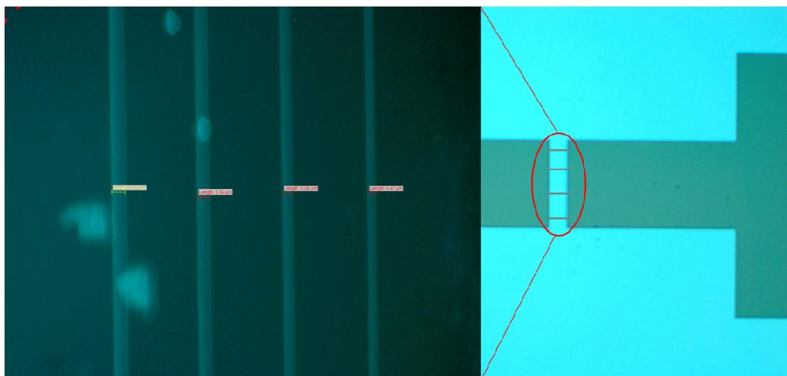
Fig. 1, HPM image fabricated silicon nanowire
