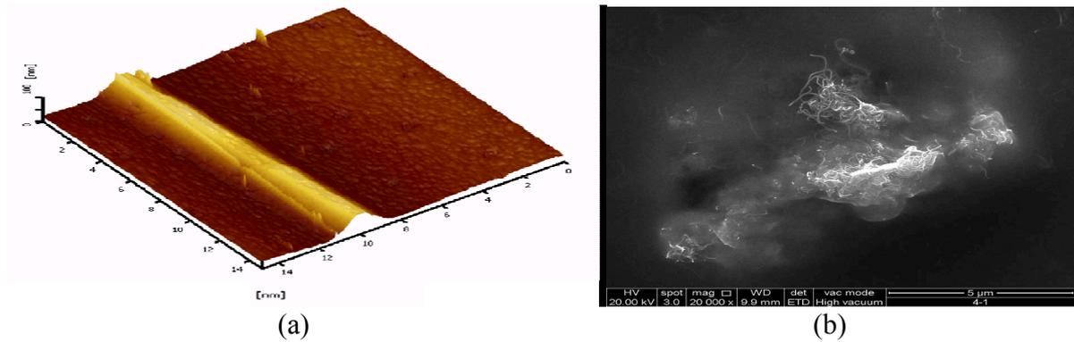
Fig. 2, (a) AFM image fabricated silicon nanowire (b) Surface modified silicon nanowire with Chitosan
