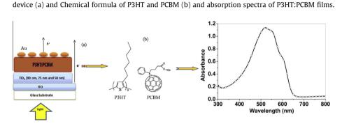
Schematic demonstration of ITO/TiO2 (different thickness/P3HT:PCBM/Au) bulk hetero junction PV
