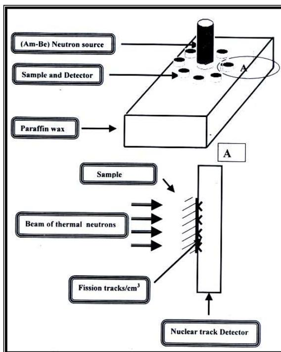
Fig.1 Shows the soil sample and detector irradiation in front of thermal neutron source
