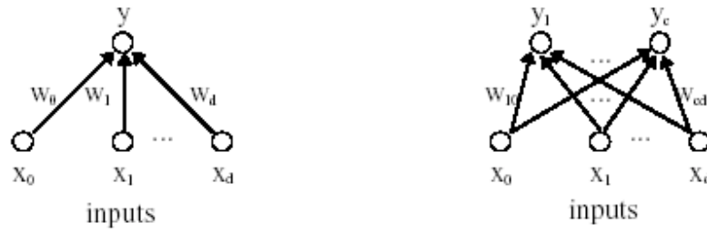
Figure 3.3 The simplest neural networks. Computation is done in the second layer of nodes
