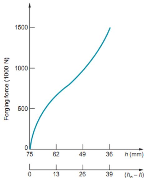
Figure 7.4 Upsetting force as a function of height  $h$  and height reduction  $(h_0 - h)$ . This plot is sometimes called the load stroke curve.
