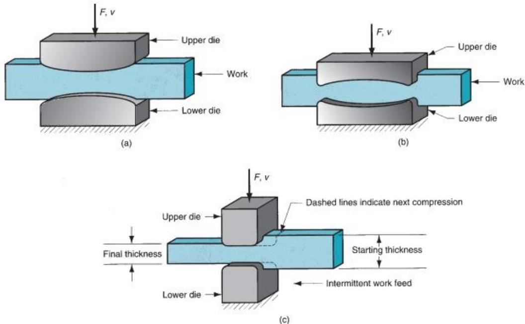
Figure 7.5 Several open-die forging operations:
