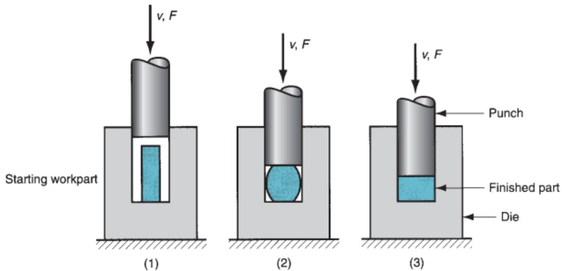
Figure 7.9 Flashless forging: (1) just before initial contact with workpiece, (2) partial compression, and (3) final punch and die closure. Symbols  $v$  and  $F$  indicate motion ( $v = \text{velocity}$ ) and applied force, respectively.
