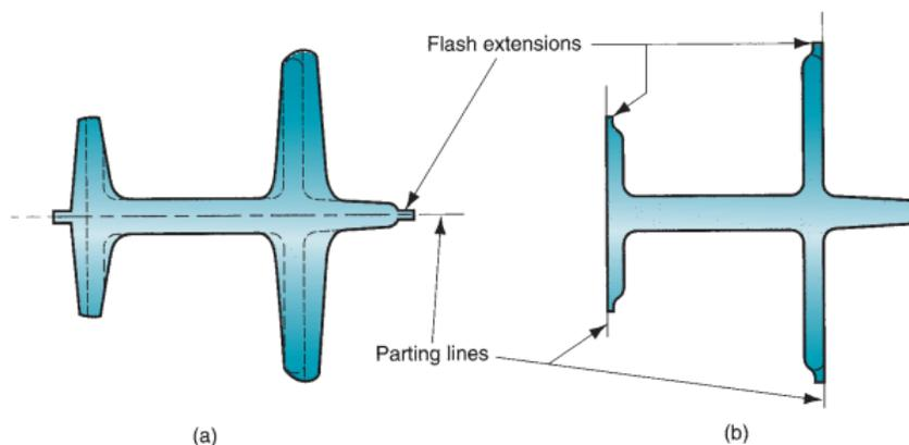
Figure 7.8 Cross sections of (a) conventional-and (b) precision forgings. Dashed lines in (a) indicate subsequent machining required to make the conventional forging equivalent in geometry to the precision forging. In both cases, flash extensions must be trimmed.
