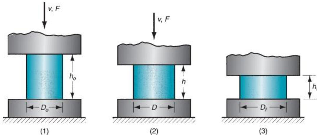
Figure 7.2 Homogeneous deformation of a cylindrical workpart under ideal conditions in an open-die forging operation: (1) start of process with workpiece at its original length and diameter, (2) partial compression, and (3) final size
