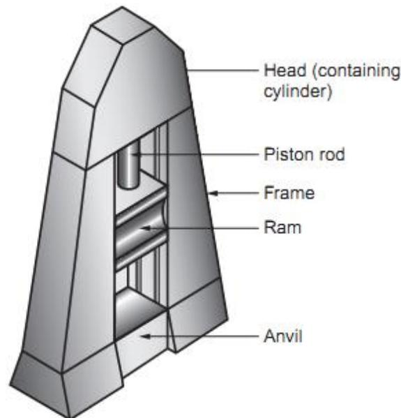
Figure 7.11 Diagram showing details of a drop hammer for impression-die forging.
