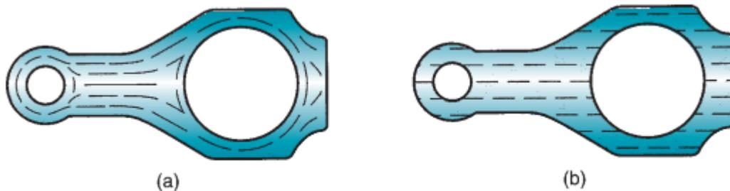
Figure 7.7 Comparison of metal grain flow in a part that is:
