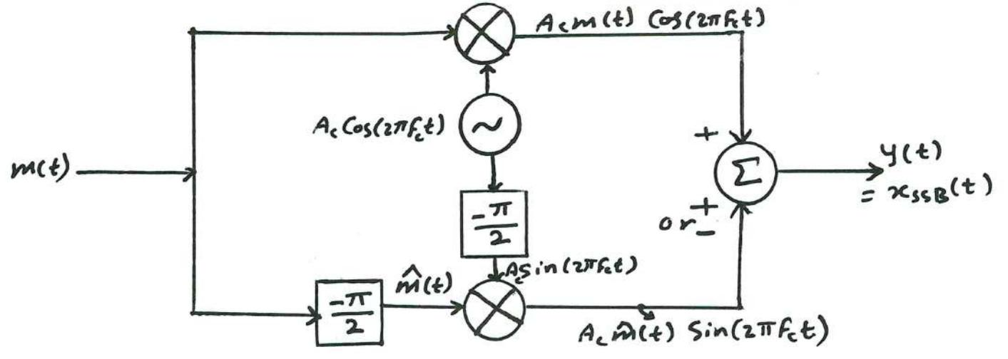
$$x_{SSB}(t) = A_c m(t) \cos(2\pi f_c t) \begin{matrix} \xrightarrow{\text{For USB}} \\ - \\ \xrightarrow{\text{For LSB}} \end{matrix} A_c \hat{m}(t) \sin(2\pi f_c t)$$
