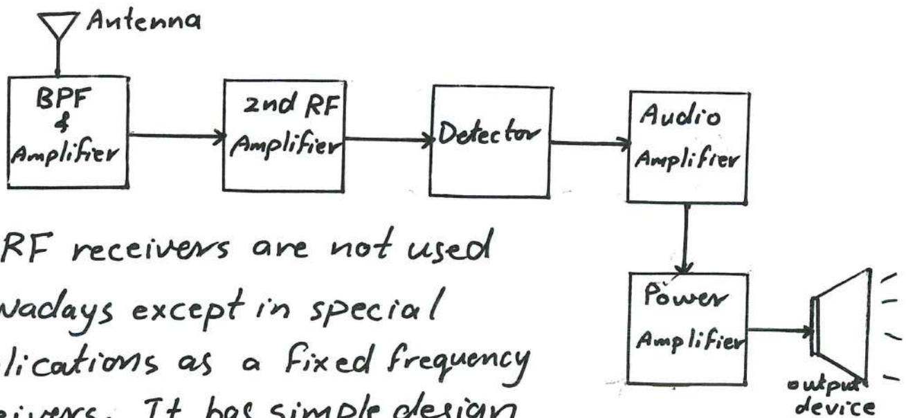
TRF receivers are not used nowadays except in special applications as a fixed frequency receivers. It has simple design but bad quality signal.
