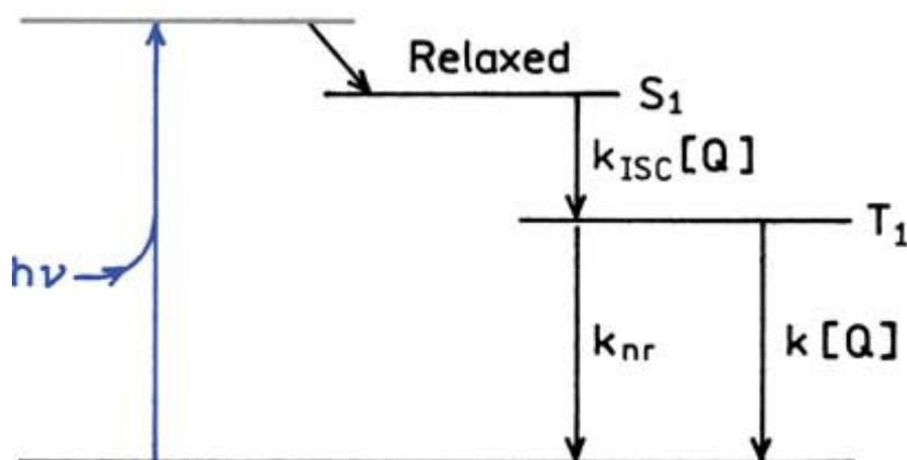
Figure 8. Quenching by intersystem crossing.
